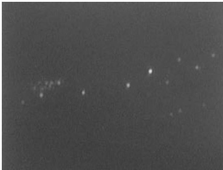
Figure 3 - Beam waist and profile as seen from the side. Light from the laser at low power is scattered off of 0.7 micron quartz spheres indicating the intensity of the laser in different regions. It is easy to see where the laser beam converges to its focus on the left end of the picture.
