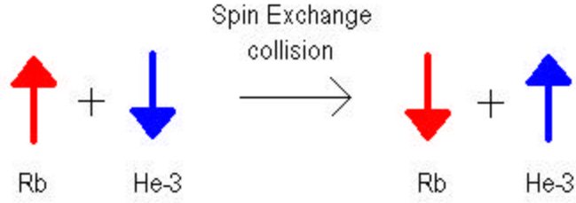
Figure 4: Rb atoms collide with ^3\text{He} atoms and transfer spin to the ^3\text{He} nuclei. This causes the Rb to depolarize, but it is quickly optically pumped into a polarized state where it is again ready for spin exchange.
