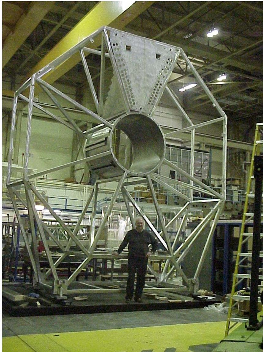
Figure 3.1. Support structure for the eight octants. Octant 7 is shown installed in the 12 o'clock position.
