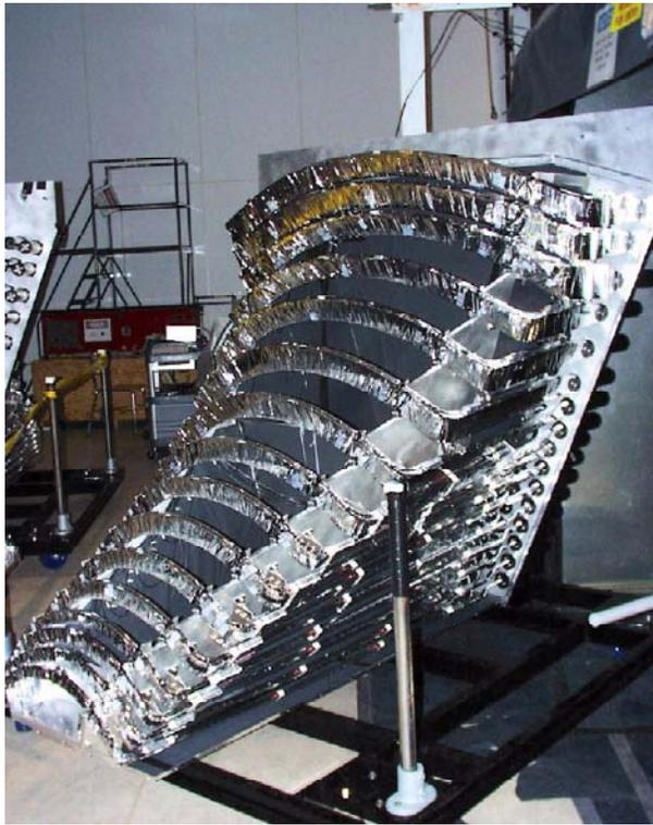
Figure 3.3. An octant comprised of 16 pairs of arc-shaped plastic scintillators. The scintillators are wrapped in aluminized mylar to prevent contaminants such as finger oils from crazing (formation of cracks and scratches) the plastic.
