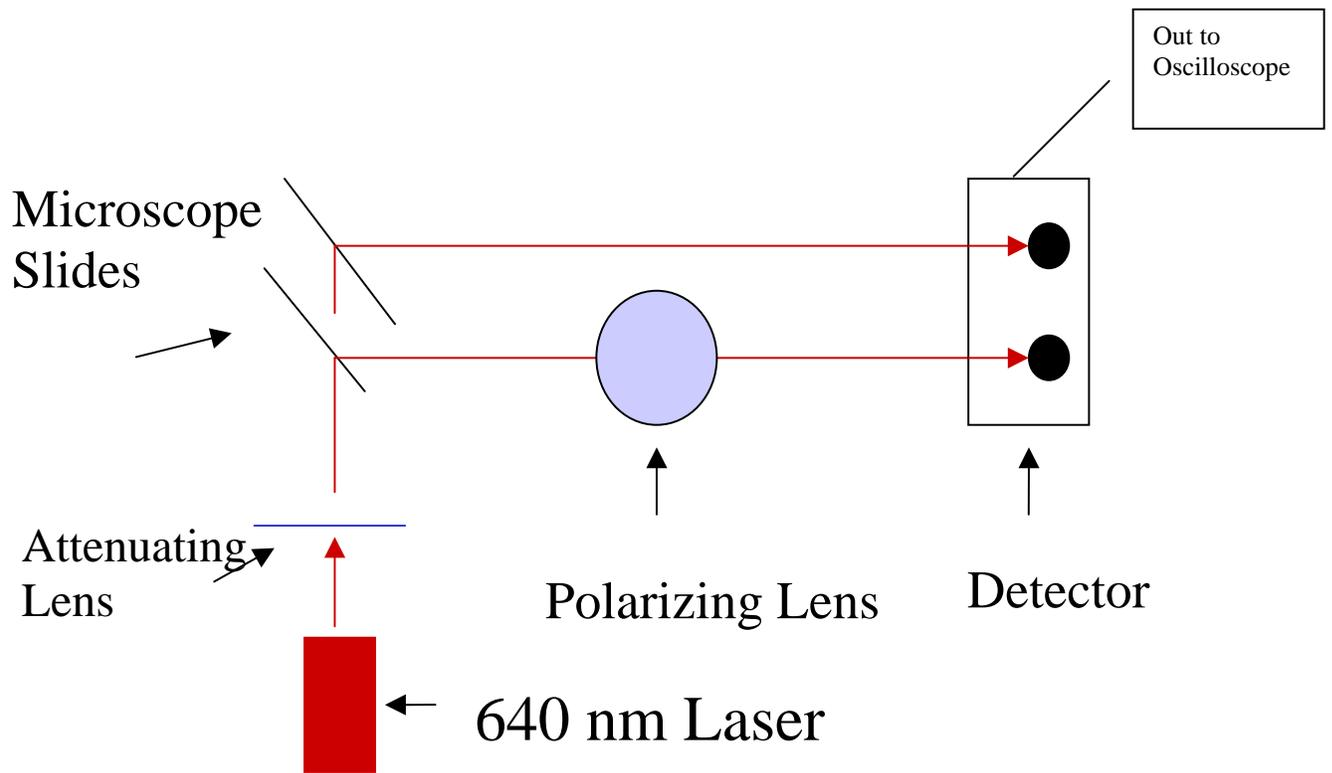
Figure 4: Single Color Laser Setup
