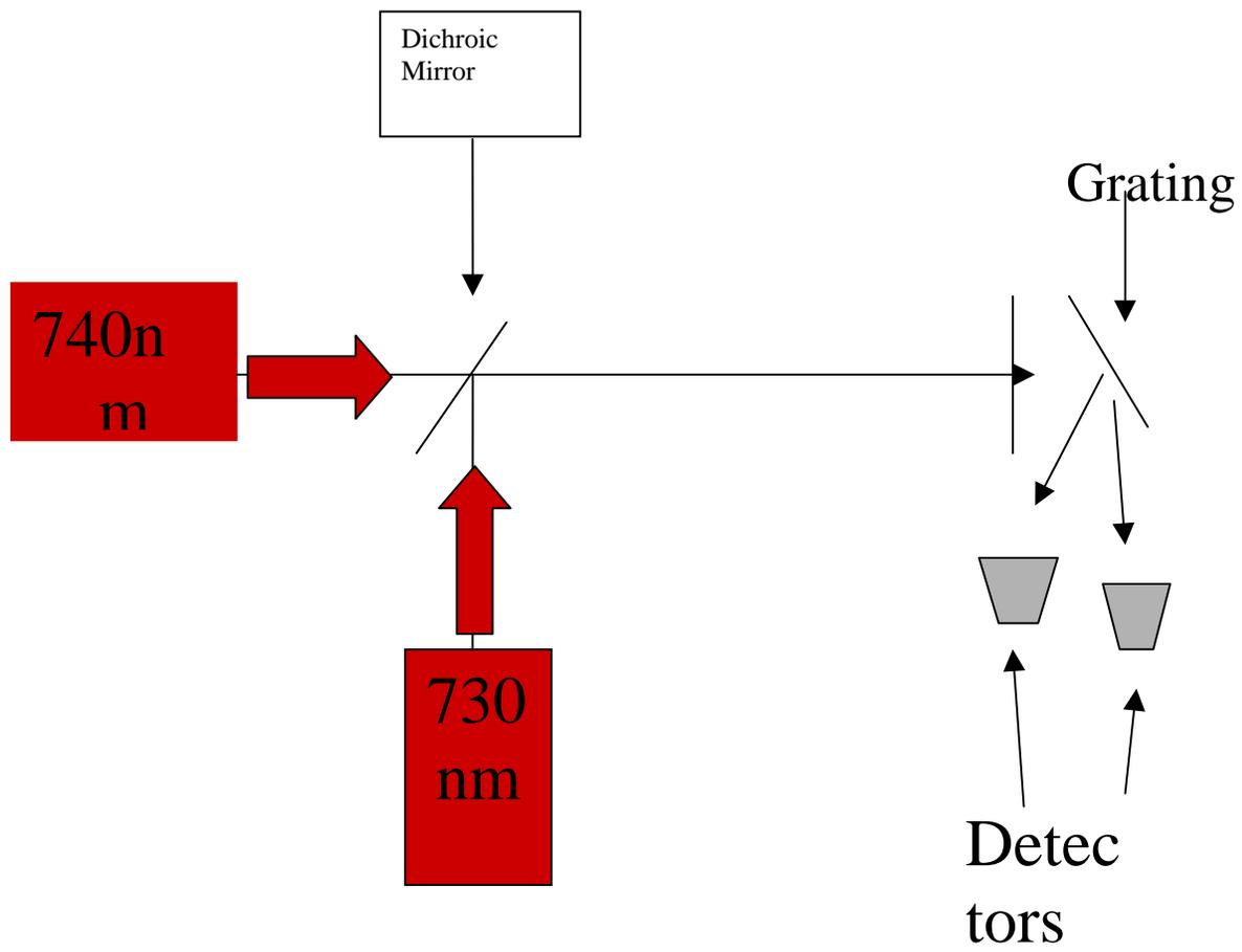
Figure 3: Possible Differential Laser Absorption setup
