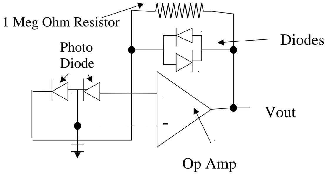
Figure 5: Electronics Setup for Light Balance Detector
