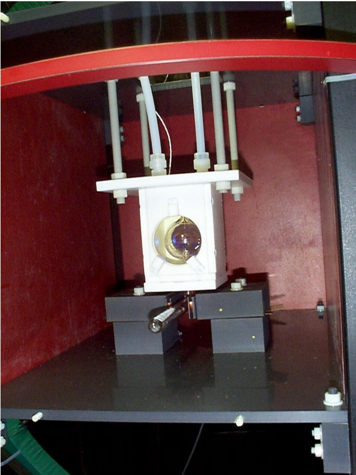
Picture 3: The oven with target cell mounted and pickup coils aligned alongside the cell.
