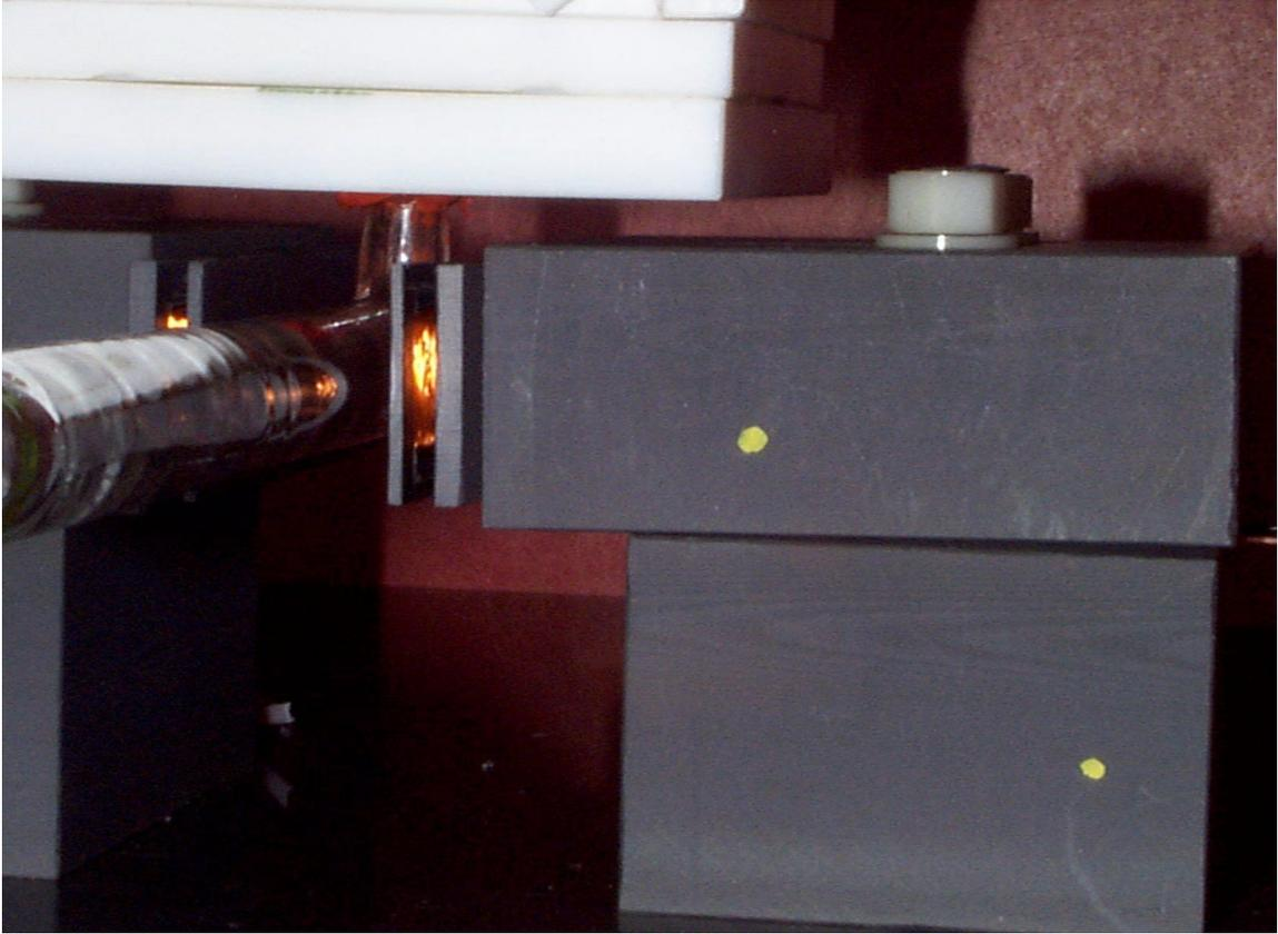
Picture 4: A side view of a pickup coil.
