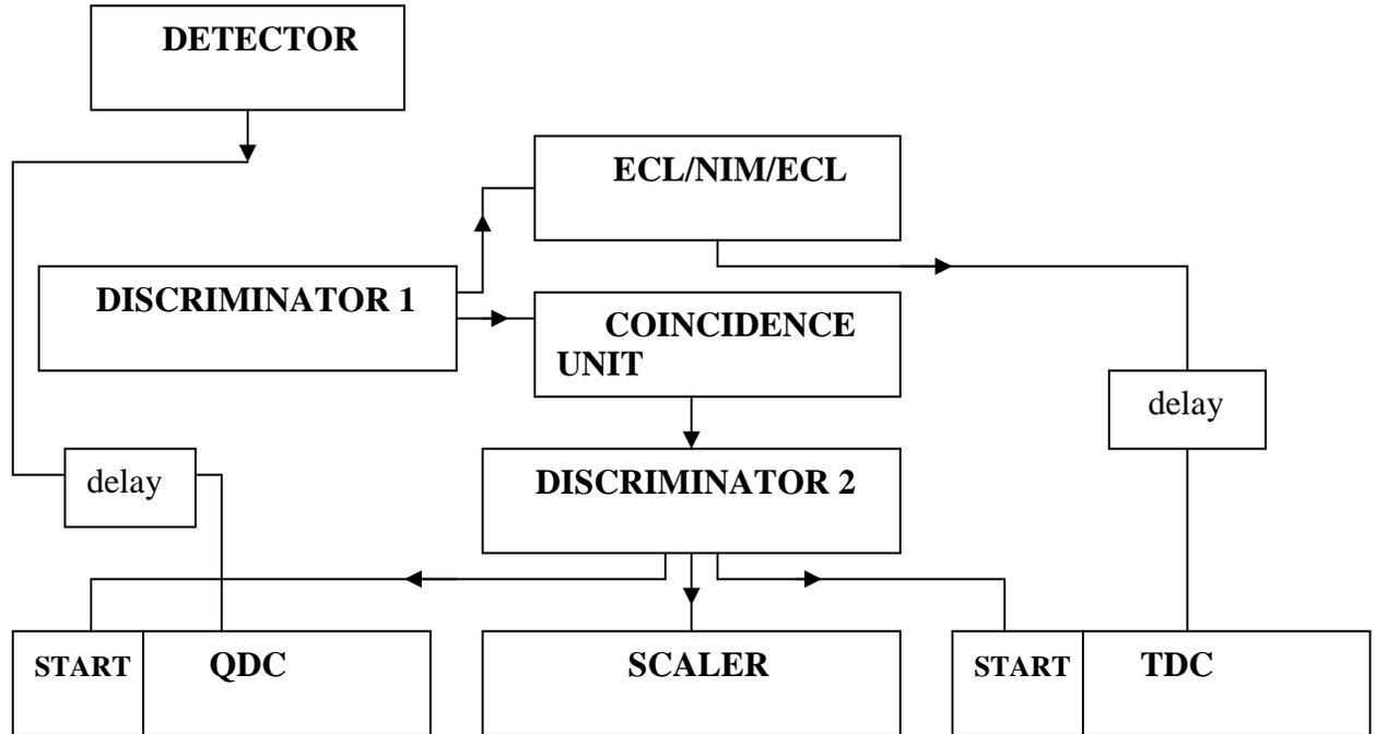
Figure 5: Detector and logic system schematic
