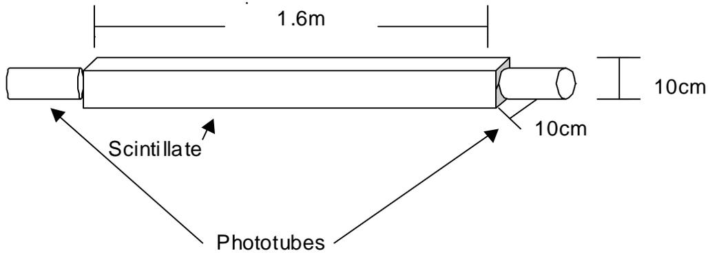
Figure 2: Scintillator and Phototube
