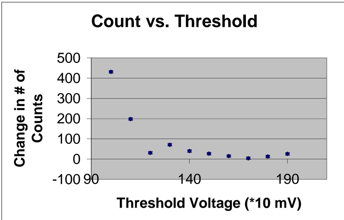
Figure 3: The change in the number of counts as the threshold voltage of the discriminator is increased. The large change for low voltages represents a large amount of noise being recorded.
