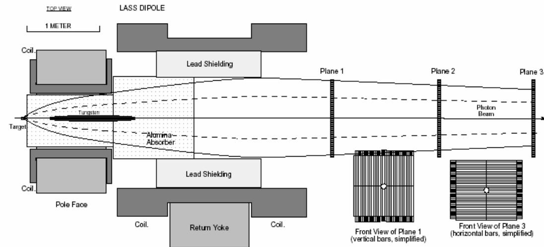
Figure 1: Spectrometer design for the SLAC E160 experiment
