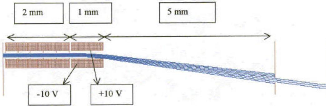
Figure 16 – Deflector Plates at 1mm
