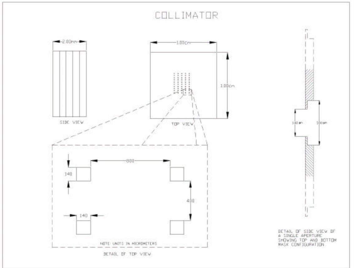
Figure 2 – The Collimator
