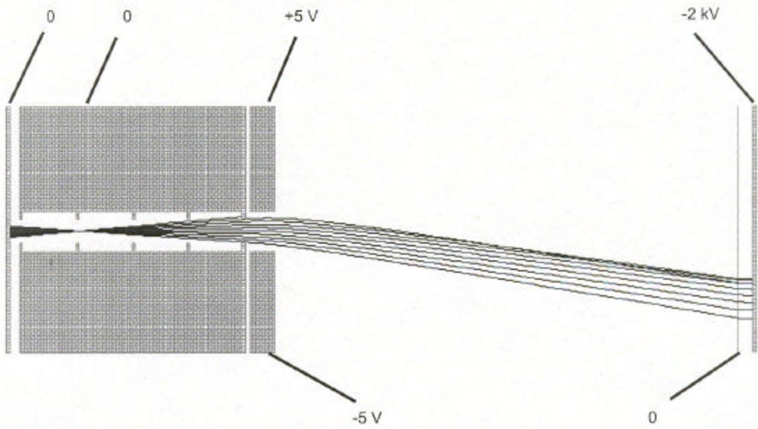
Figure 11 – Change in Kinetic Energy and Angle of Ions
