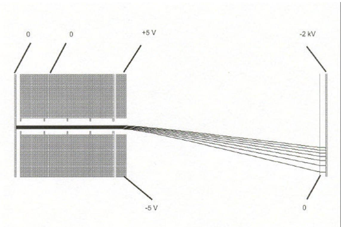
Figure 9 – Change in Kinetic Energy of Ions
