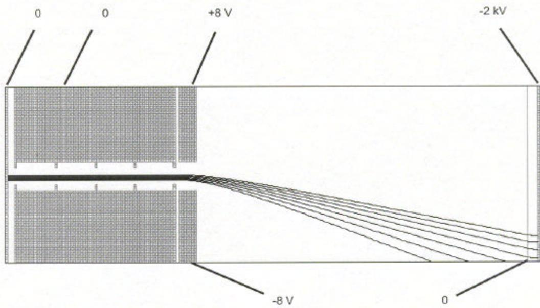
Figure 12 – Change in Kinetic Energy of Ions
