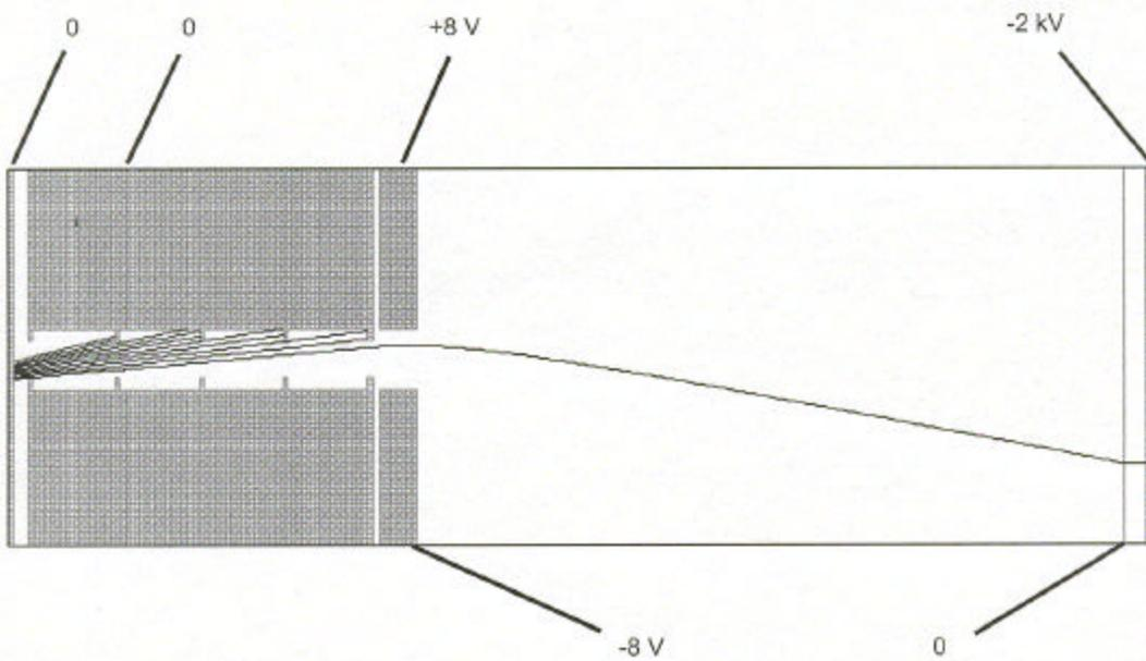
Figure 13 – Change in Initial Angle of Ions
