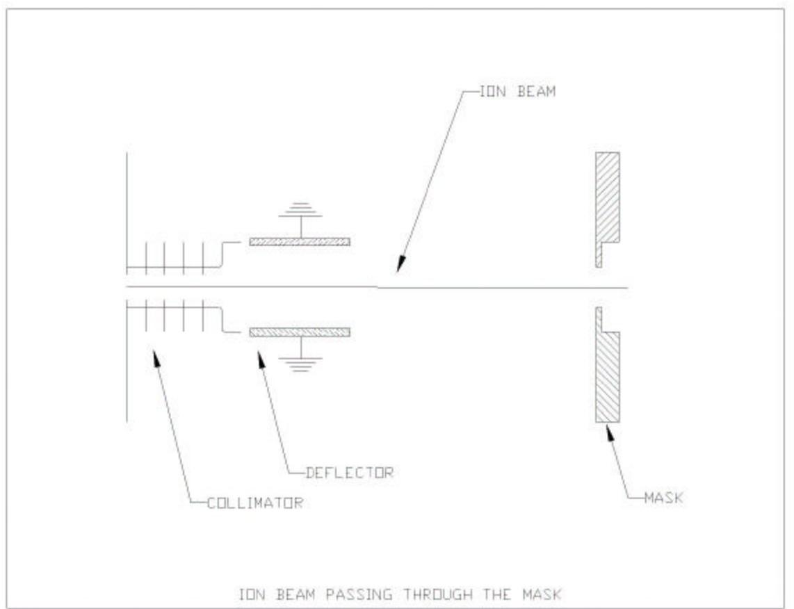
Figure 4 – Ion Beam With No Deflection
