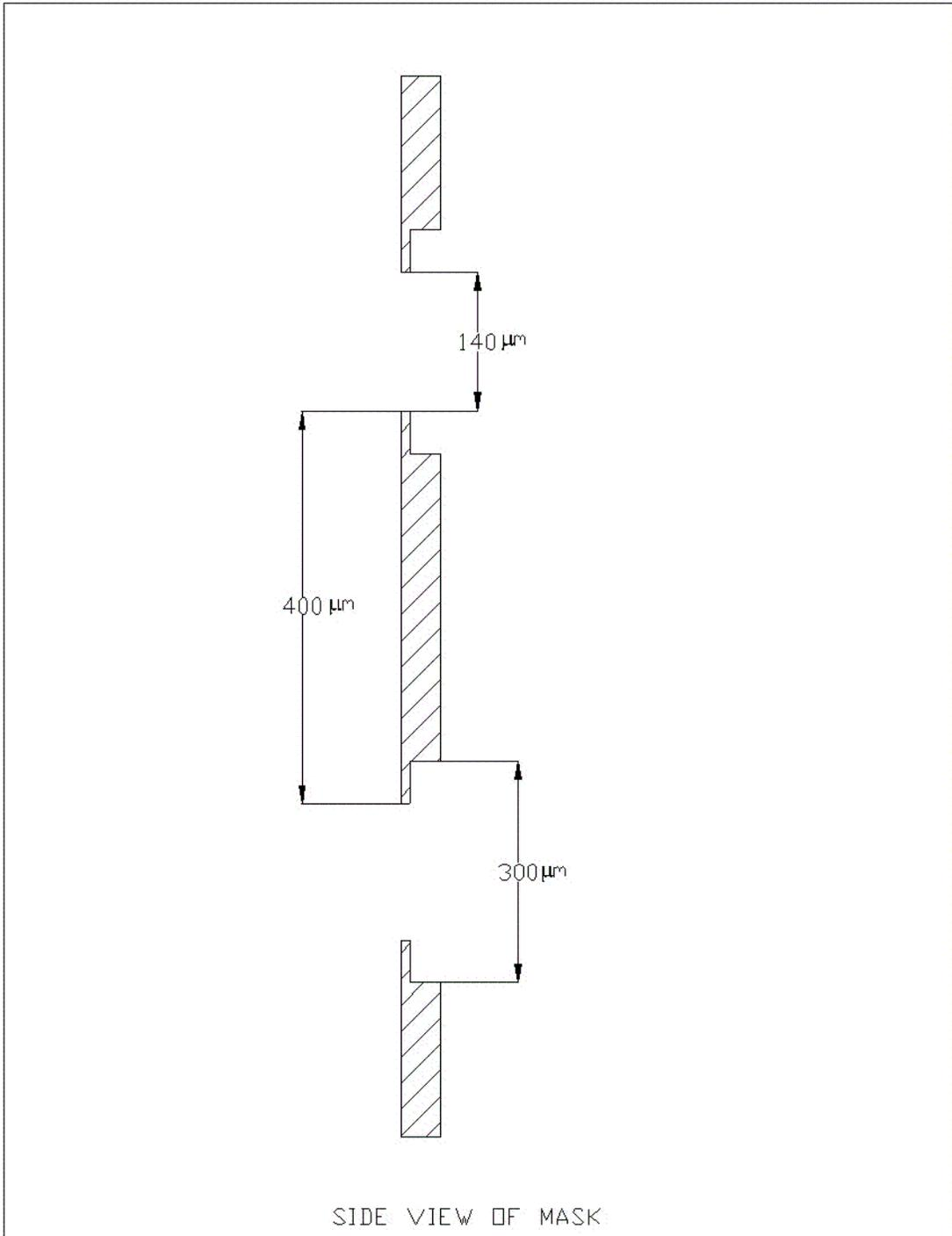
Figure 6 – Detailed View of the Mask
