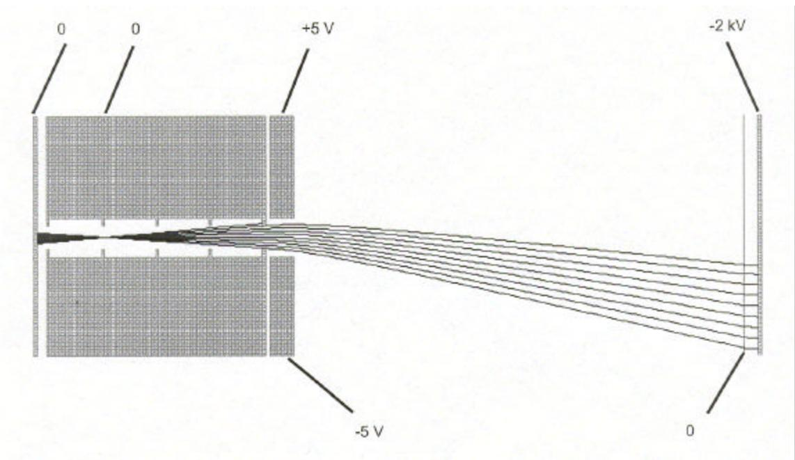
Figure 10 – Change in Initial Angle of Ions
