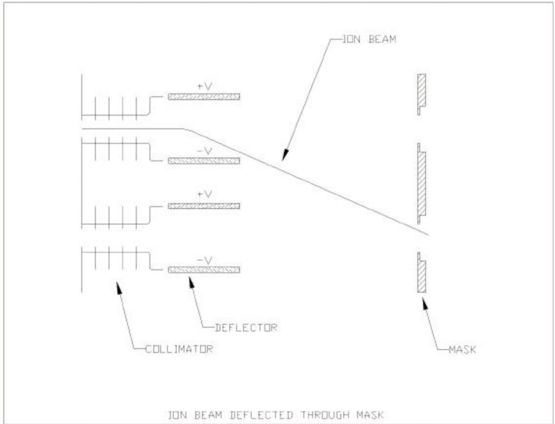
Figure 5 – Ion Beam Deflected Through Secondary Hole in Mask
