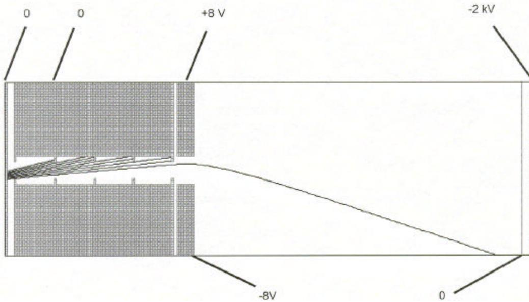
Figure 14 – Change in Kinetic Energy and Angle of Ions
