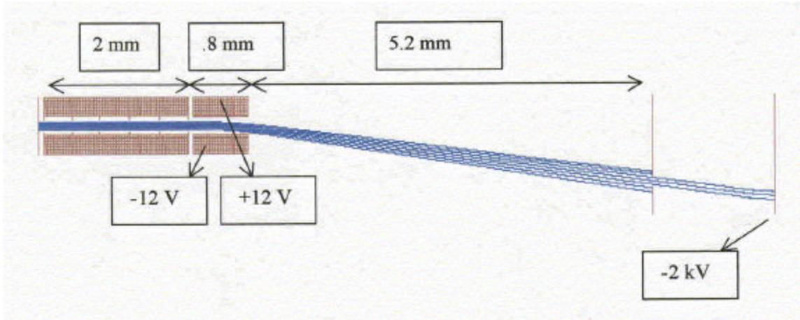
Figure 18 – Deflector Plates at 0.8mm
