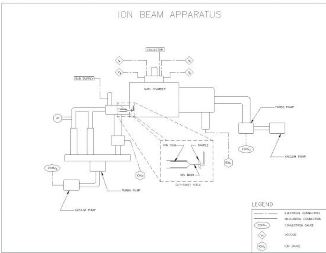
Figure 7 – Ion Beam Apparatus
