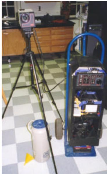
**Figure 5- Custom data acquisition cart**
