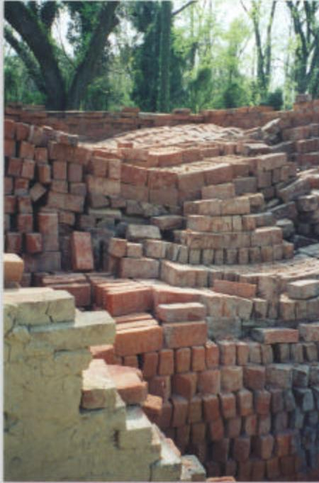
**Figure 34- Photo showing the kiln partially disassembled as the bricks are being removed and sorted for use in the spring. Note the differing colors of the bricks, denoting differences in hardness. The grayish bricks are much harder than the more salmon colored ones.**
