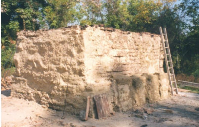
**Figure 33- Sealed up kiln cooling off**
