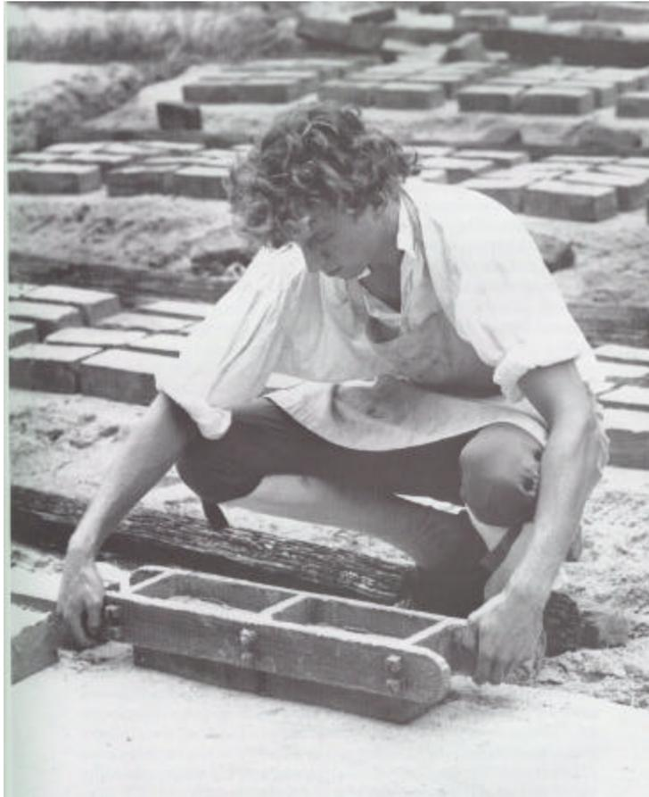
**Figure 32- "Bearing Off" the wet, or "green" bricks.<sup>30</sup>**
