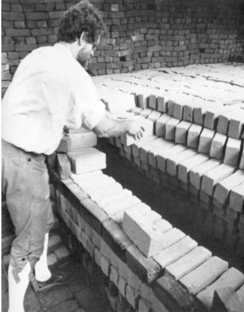
**Figure 11- Unfired bricks are stacked within the kiln with about a thumbs space between to facilitate heat flow. <sup>10</sup>**
