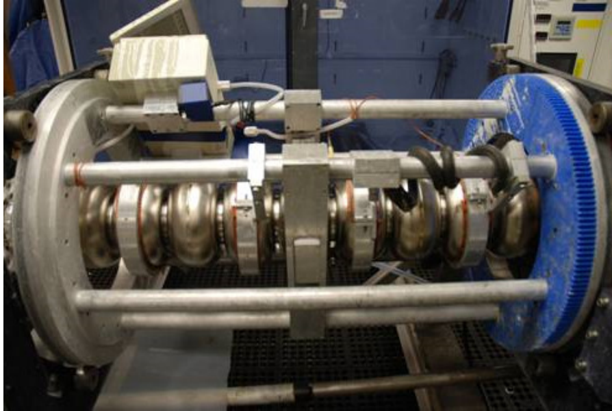
Figure 1: A superconducting RF cavity used in the particle accelerators. (Photo courtesy the Thomas Jefferson National Accelerator Facility.)
