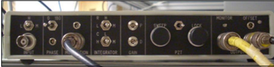
Figure 3: Lock-in amplifier LIHV200 without photodiode INPUT connection
