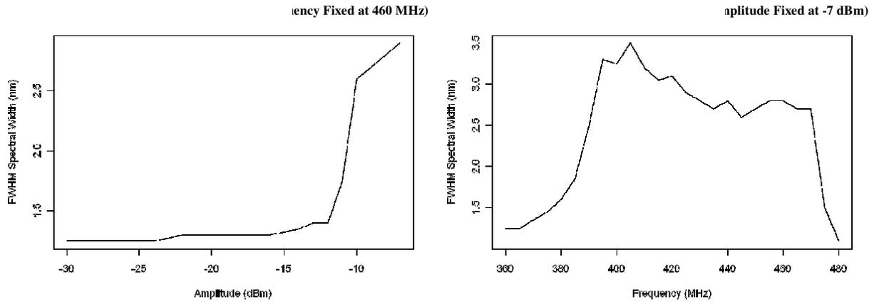
Figure 14: Amplitude Optimization of Mode-Locked Diode Laser Spectrum (Left)
