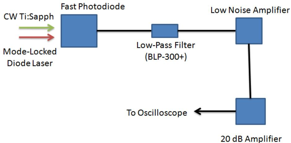
Figure 23: Circuit diagram for the filter and amplifiers.
