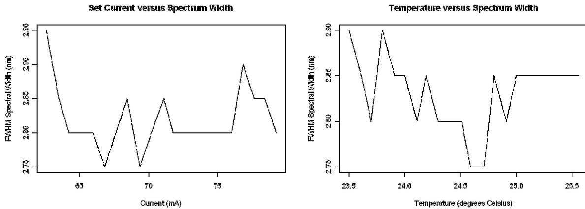
Figure 15: Set Current Optimization of Mode-Locked Diode Laser Spectrum (Left)
