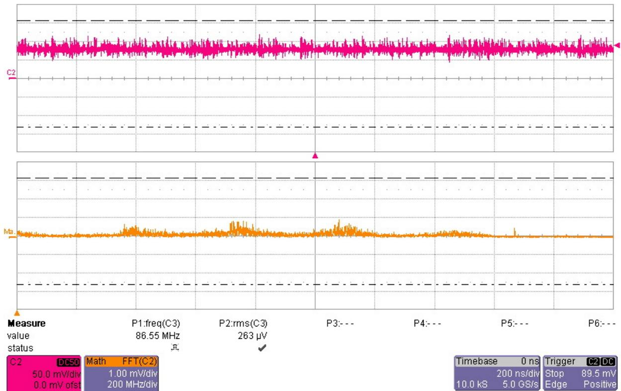
Figure 27: Noisy signal that appears to be caused by the diode laser entering into passive mode-locking. This was prevented by adjusting the aperture in the laser cavity until the signal was gone.
