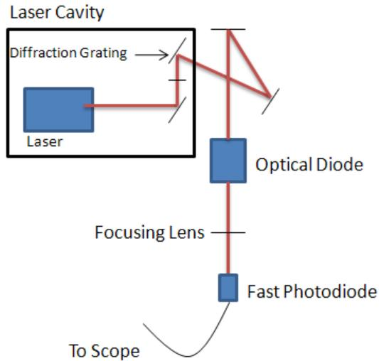
Figure 5: Setup used to verify active mode-locking
