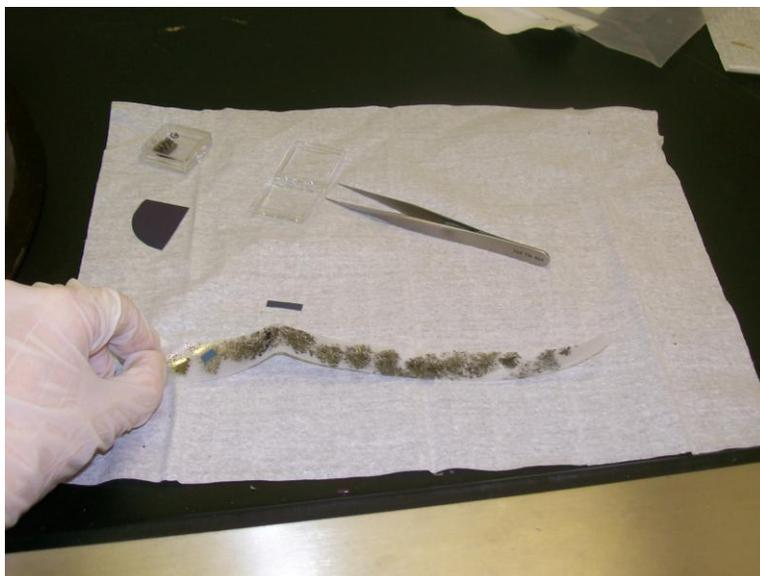
**Figure 9: Adhesive “Scotch” tape after being pressed to the HOPG and folded over several times upon itself.**
