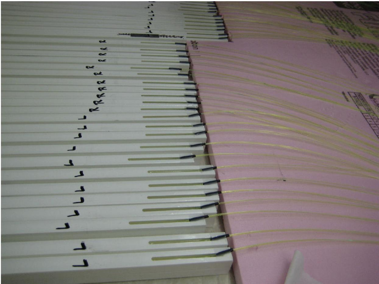
*Figure 1: This image shows MINERvA outer detector scintillators lined up next to each other. The white color on the outside is given by the titanium dioxide coating for reflectivity. The fibers coming out of them are the wavelength shifting fibers which run axially through the scintillators.*
