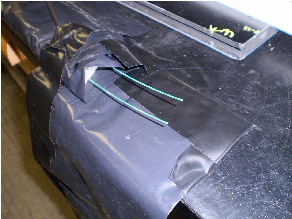
*Figure 17: A PCAL scintillator in the plastic wrap with two WLS fibers coming out. Once these fibers are connected to the extension cable the plastic underneath it will be wrapped around it and taped in place to ensure that it is light-tight.*
