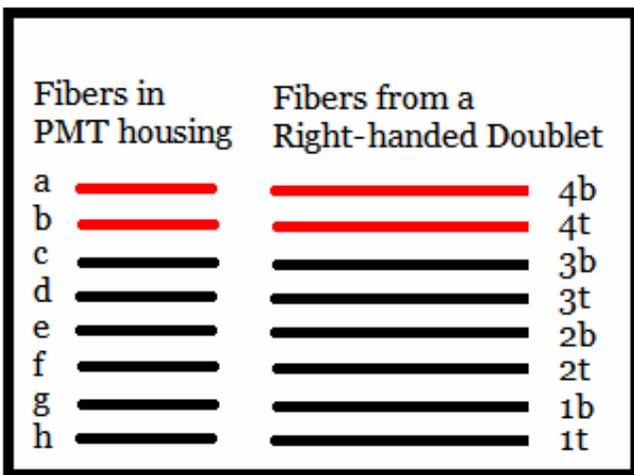
Figure 7: Diagram of fiber connections in the testing apparatus.
