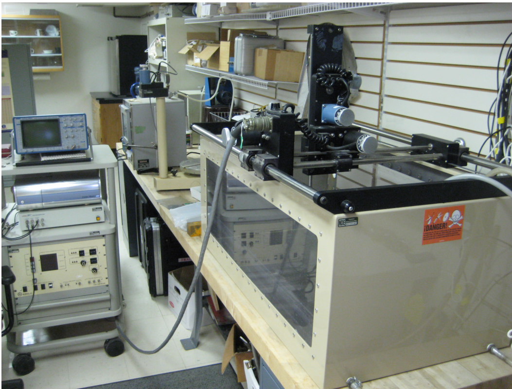
Figure 22: Ultrasonic immersion tank used to scan flawed and control chips for confirming our results. The process is automated and computer controlled.
