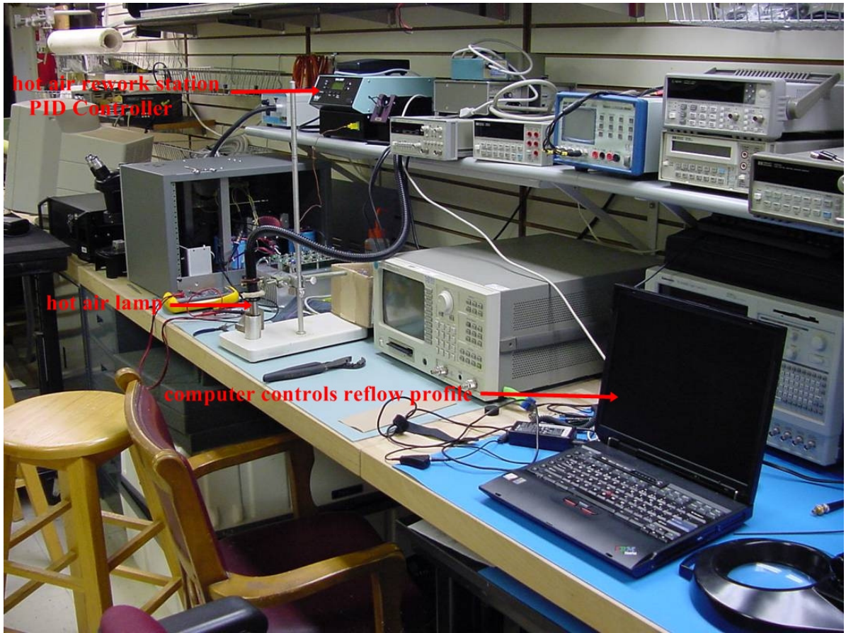
Figure 8: Reflow profile apparatus. Computer controls hot air lamp, which heats IC's to 260°C to simulate the shock of soldering.
