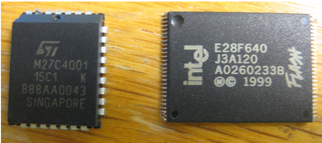
Figure 10: Integrated circuits we performed our research on. We scanned 12, 32 pin PLCCs (pictured left) and 12, 56 pin TSOPs (pictured right)
