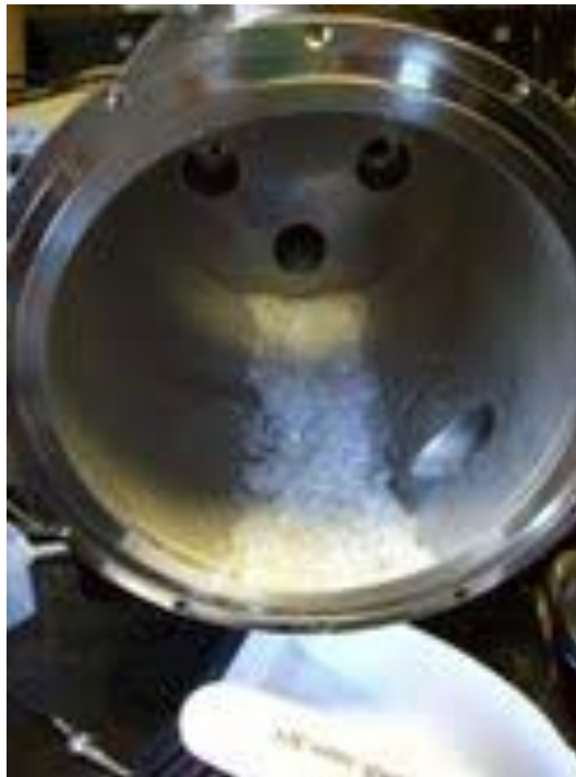
Figure 11: William and Mary Cell # 3 after cell burst and ^3\text{He} recovery.
