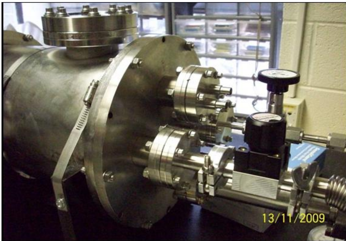
Figure 8: Right side of the chamber. Seen here are: at top of faceplate, the BNC feed through; on the left, valve which goes to the roughing pump; on the right, valve to ^3\text{He} holding tank; not seen, but on the bottom, nipple for the target chamber of the cell to rest in. On the top of the chamber is the viewport.
