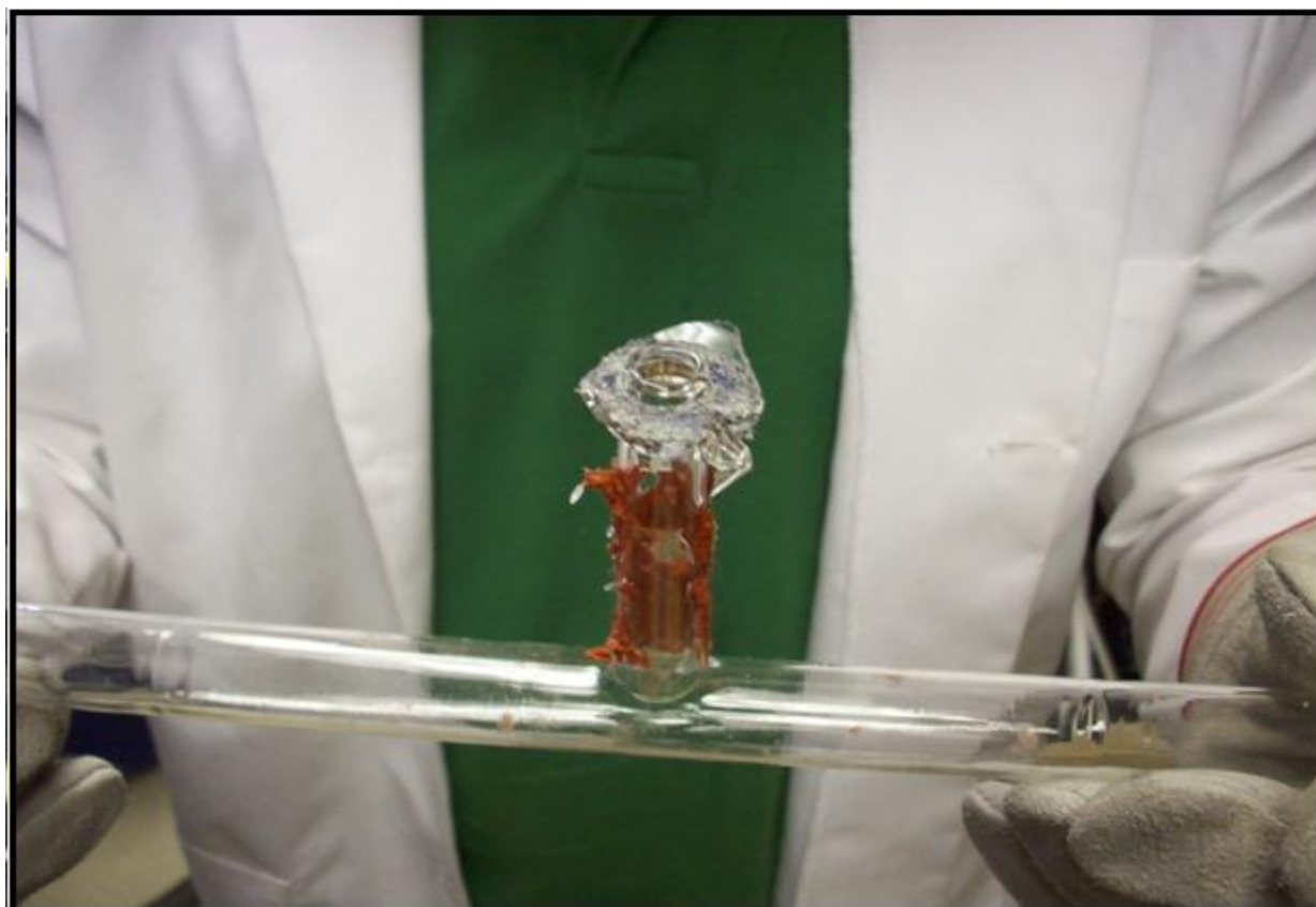
Figure 10: William and Mary Cell #2. The pumping chamber exploded during solenoid impact.
