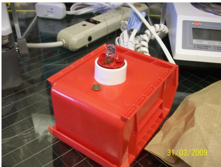
Figure 14: Constructed lightbulb holder with light bulb without glass bulb for the light bulb test
