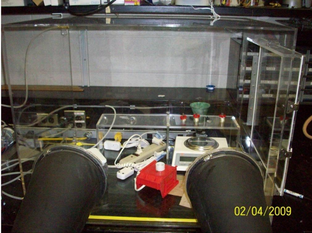
Figure 19: Glovebox front view under pressure
