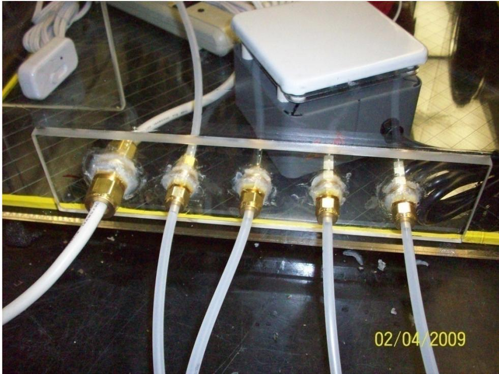
Figure 17: Glovebox feed-throughs with connections
