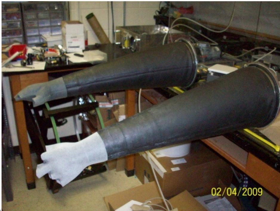
Figure 18: Glovebox under pressure
