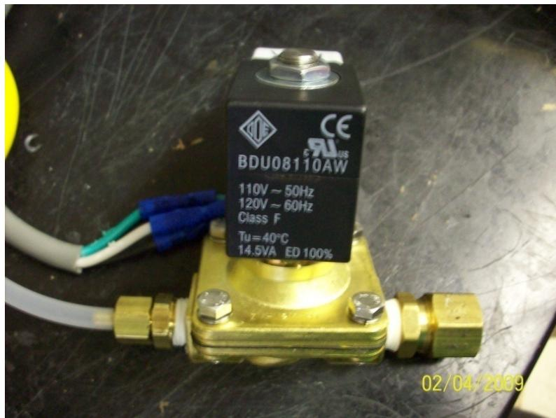
Figures 9: Solenoid exhaust valve with relay connections, compression fit plastic tubing from box and atmospheric opening
