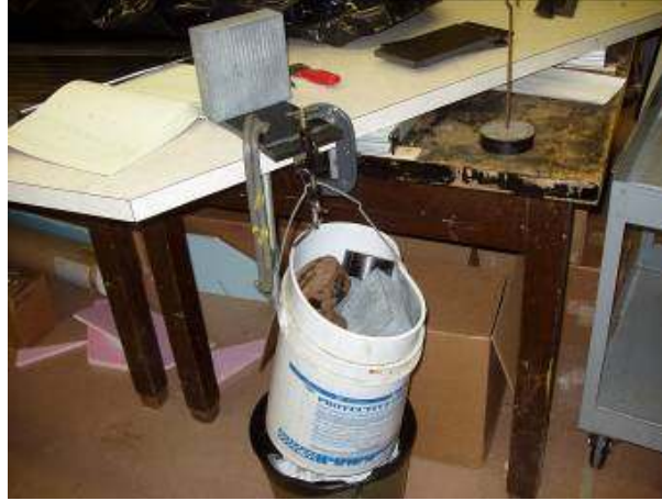
Figure 7: Weights were added to the bucket until the test sample broke.
