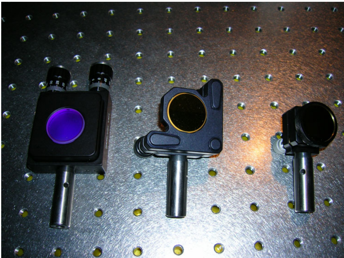
Figure 3: From left to right, the good, medium, and bad mirror mounts. All mounts are from Thor labs, and their model numbers are, from left to right, VM1, KM100, and KMS.
