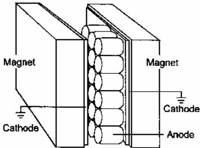
Figure 9: Ion pump in action below. The electrons from the cathode are repelled away through the anode region where they create ions that are attracted to and eventually embedded in the cathode's getter material.
