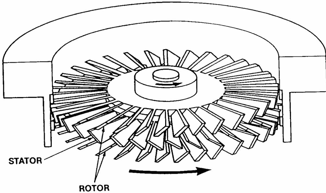
Figure 7: Turbo-molecular pump for pumping at high speeds of approximately 16000 rpm.
