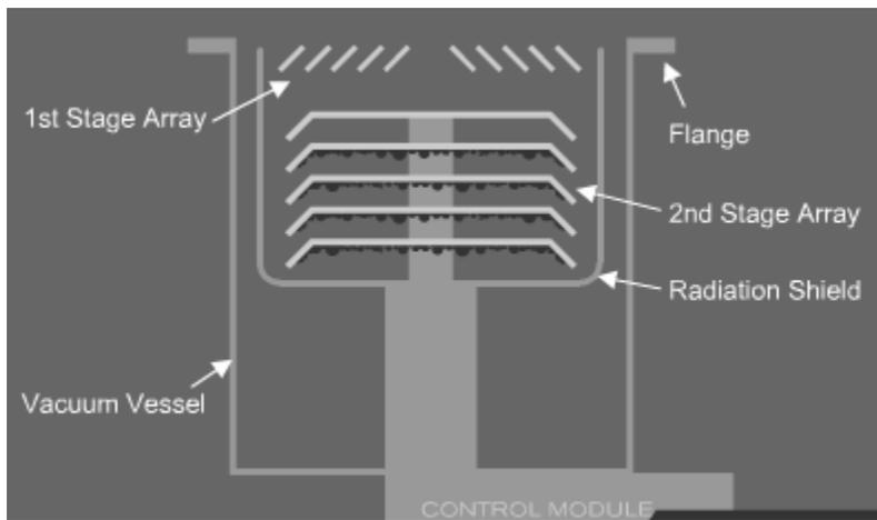
Figure 11: Activated carbon sieve attached to the second stage array for use in capturing hydrogen, helium, and neon.
