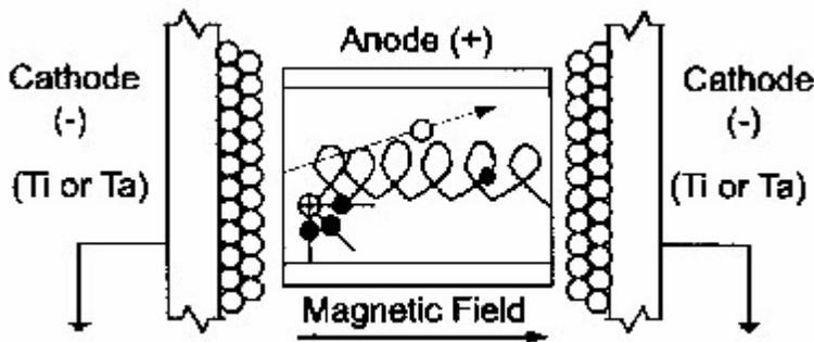
Noble diode pumps replace one of the Ti plates with Ta, which reduces the pump's H<sub>2</sub> pumping speed while allowing for better pumping of noble gases. Electrons from the cathode plates move along helical trajectories in the magnetic field through the anodic tubes.
