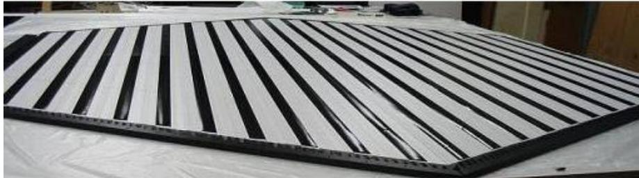
Figure 4: The weaving of the Lexan material through the array of triangular scintillator. The picture above shows a representation of how the Lexan relates to the ID scintillator strips, while the picture below shows the Lexan actually weaved through the whole plane. This picture does not show the top Lexan skins.
