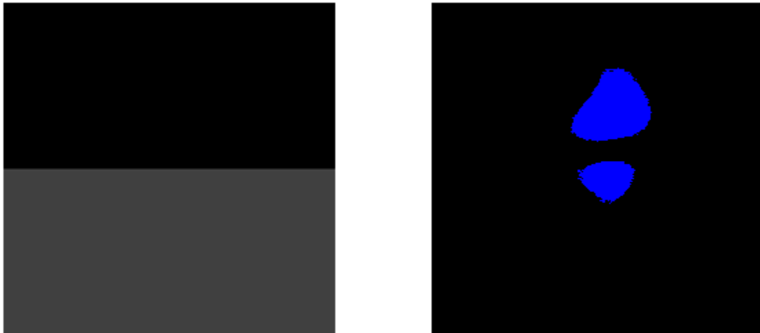
Fig. 10: A 0/64 Phase Image (left) is written to the SLM and results in a two-spot focal image (right) captured by the CCD camera.
