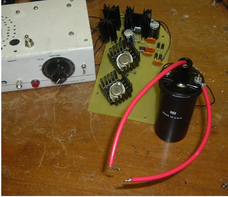
Fig. 9: Photograph of completed triggerable spark generator on prototype board with controls and spark coil.
