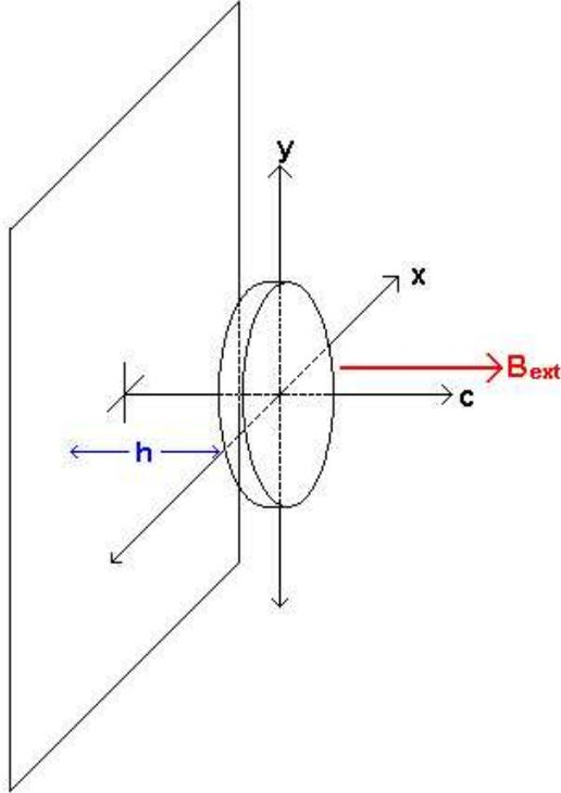
Figure 3: Model diagram of the sample, container backing material, and applied magnetic field.
