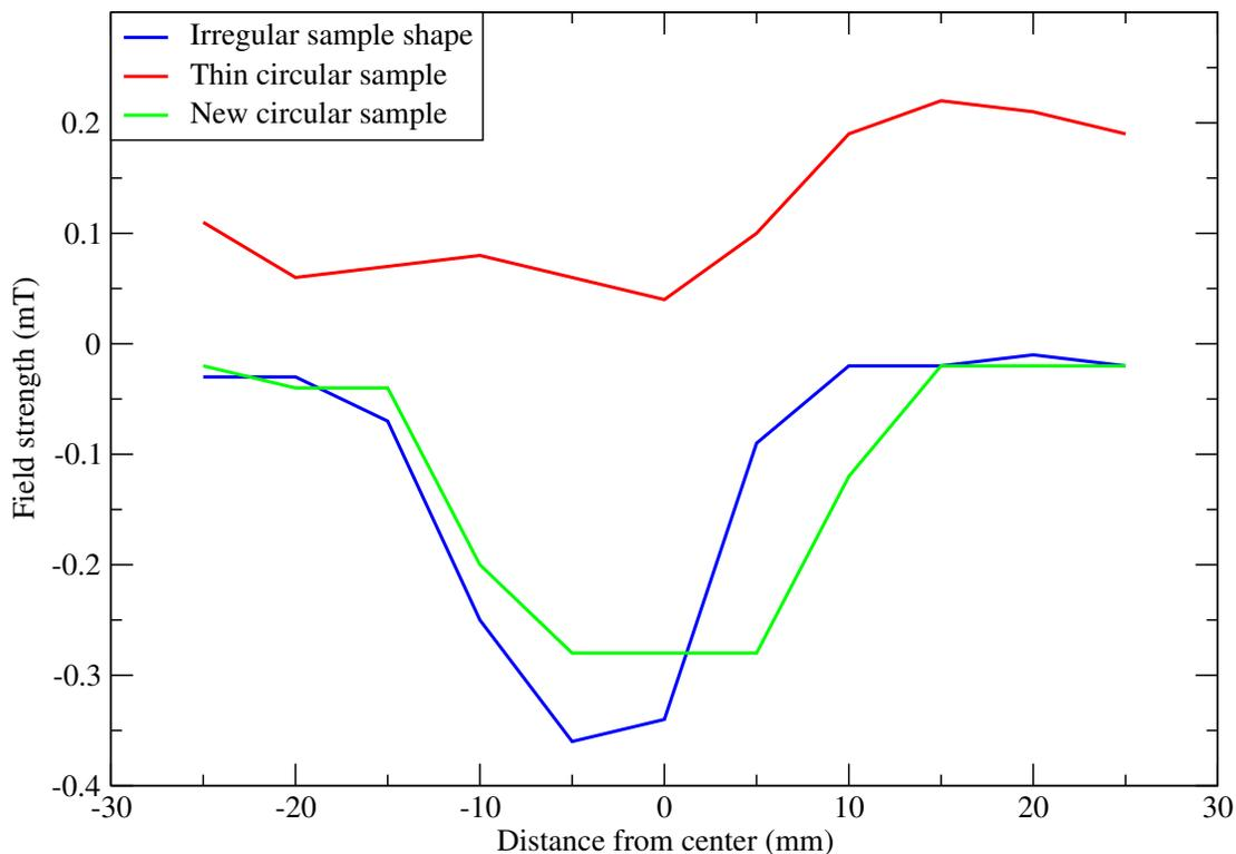
Figure 8: Surface fields of three sintered YBCO samples field-cooled in 220mT perpendicular to the circular plane.
