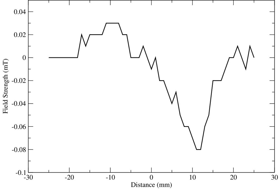
Figure 7: Surface fields of a circular sintered YBCO sample field-cooled in 220mT parallel to the circular plane.
