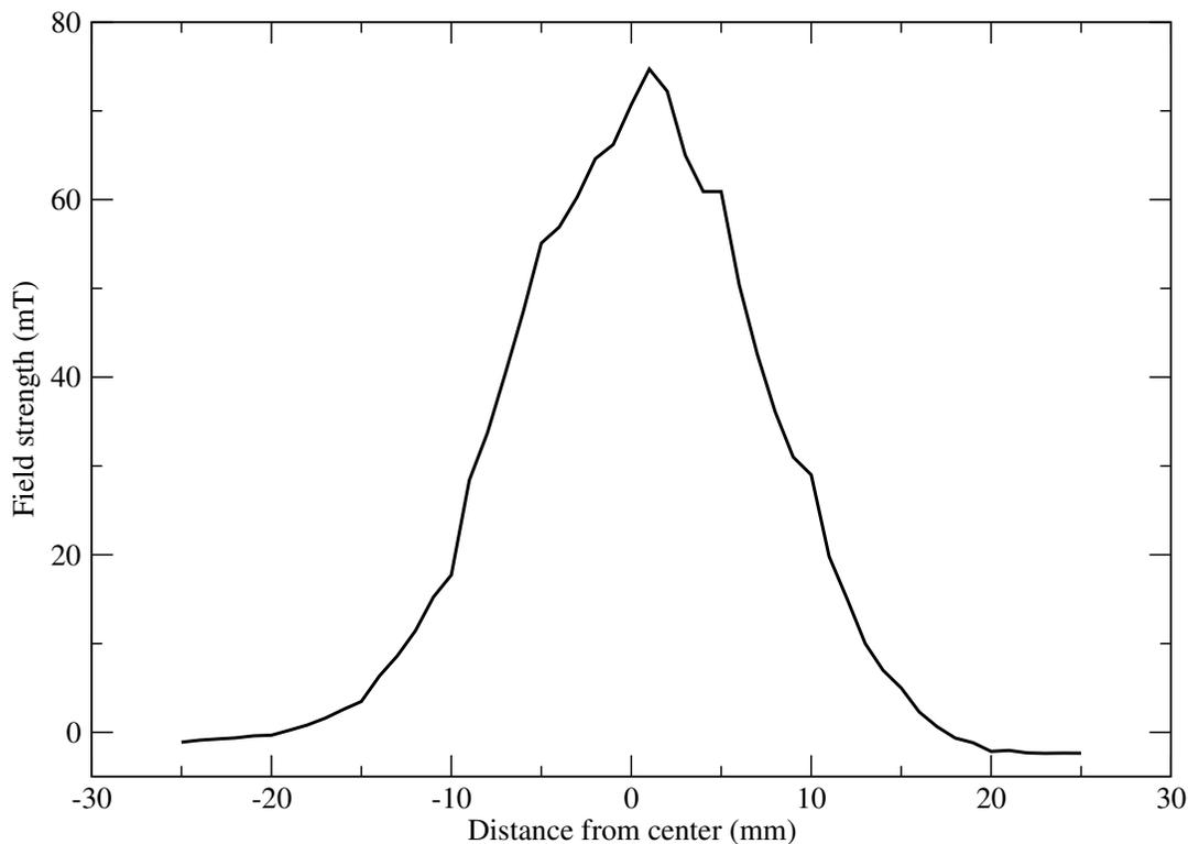
Figure 9: Surface fields of a hexagonal single-crystal YBCO sample field-cooled in 220mT perpendicular to the crystalline plane.
