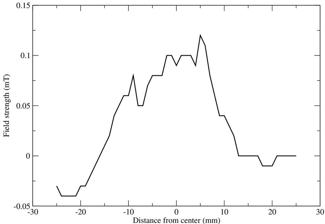
Figure 6: Surface fields of a circular sintered YBCO sample field-cooled in 220mT perpendicular to the circular plane.
