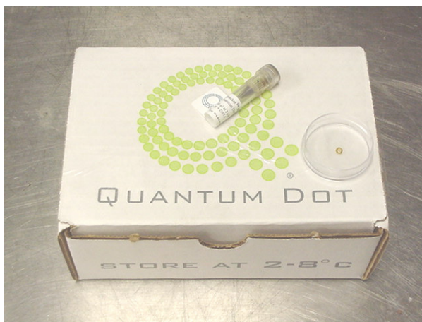
Figure 8: vial with 190 \mu\text{L} QTracker™ 800 Non-targeted quantum dots, and 10 \mu\text{L} “dot” in Petri dish (right) used for test images (200 \mu\text{L} total).
