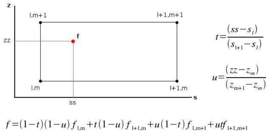
Figure 5: Interpolation Equation. This interpolation equation solves for the value at coordinate point  $f$  if the value at four surrounding points are known. ElectronPath uses this equation to solve for the drift velocity at any point within the detector using the drift velocity map at the indexed points.
