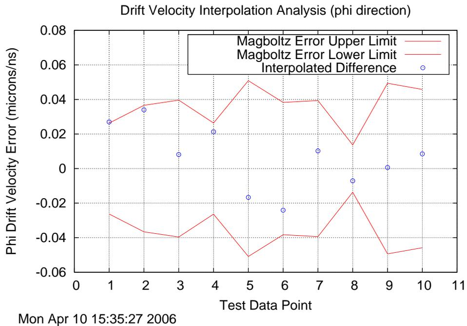
Figure 7: Interpolation Verification:  $\phi$  direction. The mean Magboltz error was  $0.0366 \frac{\mu m}{ns}$  while the mean interpolated error was  $0.0062 \frac{\mu m}{ns}$ . Since most interpolated errors lie within or very near the Magboltz error range, we can use the interpolation calculation with the current drift velocity map size without contributing significantly to the error.
