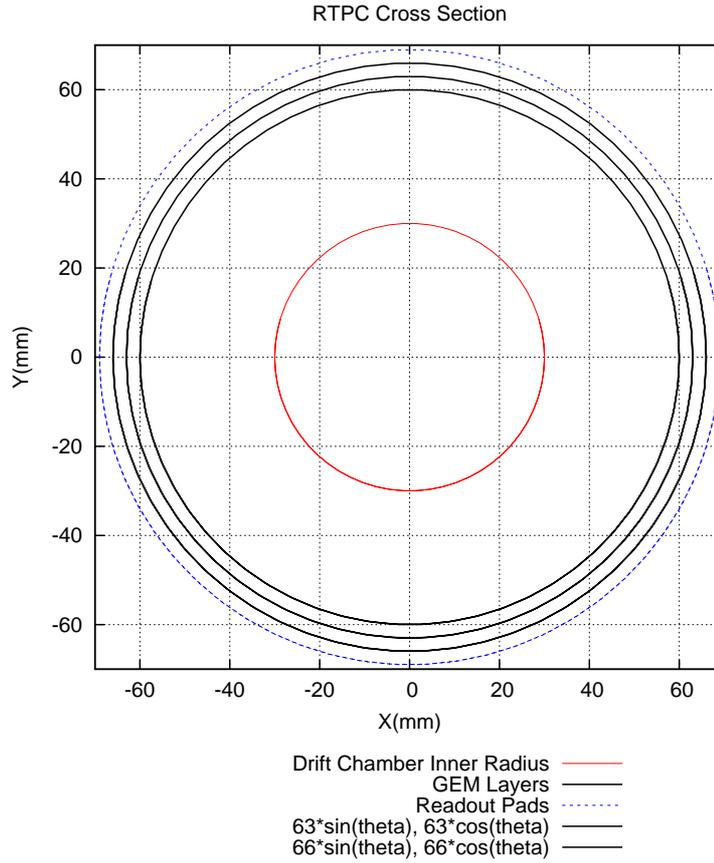
Figure 2: Cross Section of the Radial Time Projection Chamber. The inner radius of the sensitive volume is at  $s=30$  mm, GEM 1 is at  $s=60$  mm, GEM 2 is at  $s=63$  mm, GEM 3 is at  $s=66$  mm, and the readout pads are at  $s=69$  mm.
