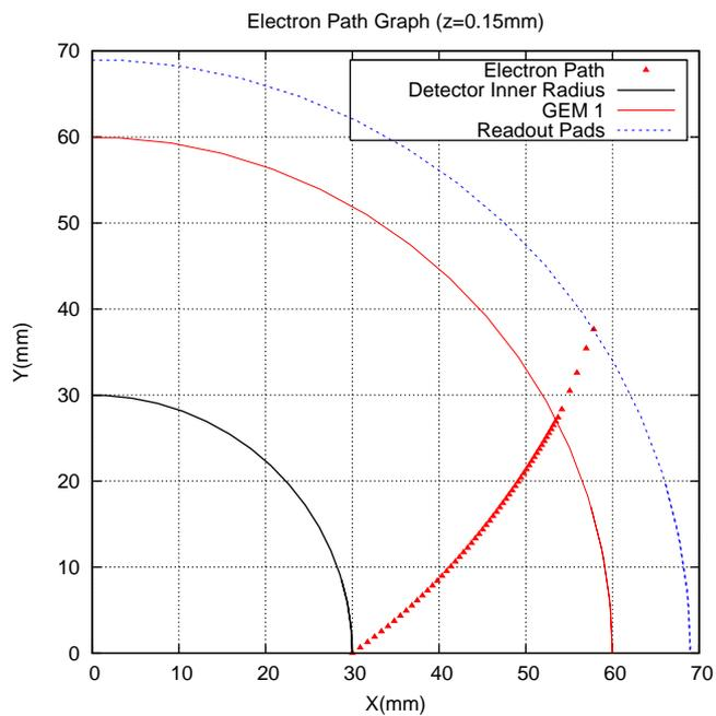
Figure 8: Electron path plot for  $z=0.15$  mm. Note that this path has more curvature than the path at  $z=98.15$  mm because the magnetic field in the  $z$  direction is stronger creating a larger Lorentz force.
