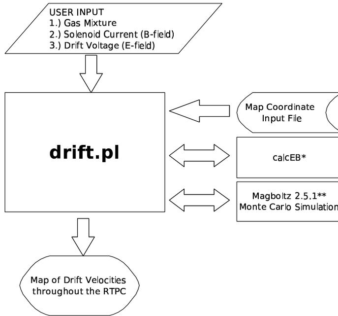
Figure 4: Drift.pl flow chart. The user is first prompted for the gas mixture, solenoid current, and the RTPC voltages. The map coordinate input file gives drift.pl the coordinate points for which the drift velocity information will be calculated. The program then runs calcEB and Magboltz 2.5.1 for each coordinate point and captures the output. The drift velocities are then stored in a file named for the input parameters. This output file is the drift velocity map.
