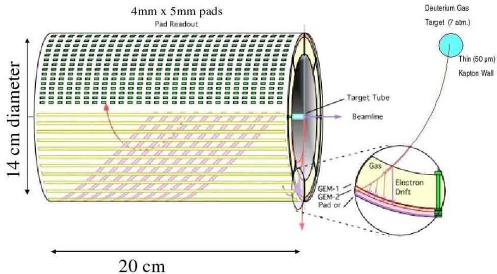
Figure 1: Dimensions and main features of the Radial Time Projection Chamber. The RTPC is 20 cm long and 14 cm in diameter. The target is a thin-walled Kapton tube 12 mm in diameter filled with 7 atm of deuterium. The target tube and sensitive volume ( $30 \text{ mm} < s < 69 \text{ mm}$ ) are shown in cross section with a schematic of an ionizing proton track and the corresponding ionization electrons.
