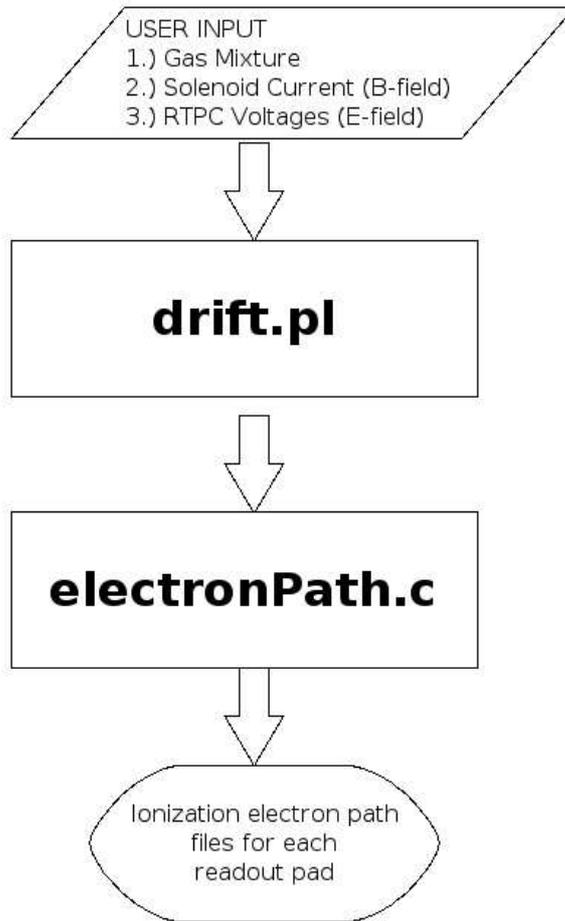
Figure 3: Program overview flow chart. Drift.pl prompts the user to input the gas mixture, the solenoid current, and the RTPC voltages. The user then runs electronPath and must input the same information. This is necessary for electronPath to find the correct drift velocity map created by drift.pl. ElectronPath then outputs a set of path files that describe the trajectory an ionization electron would travel through the detector.
