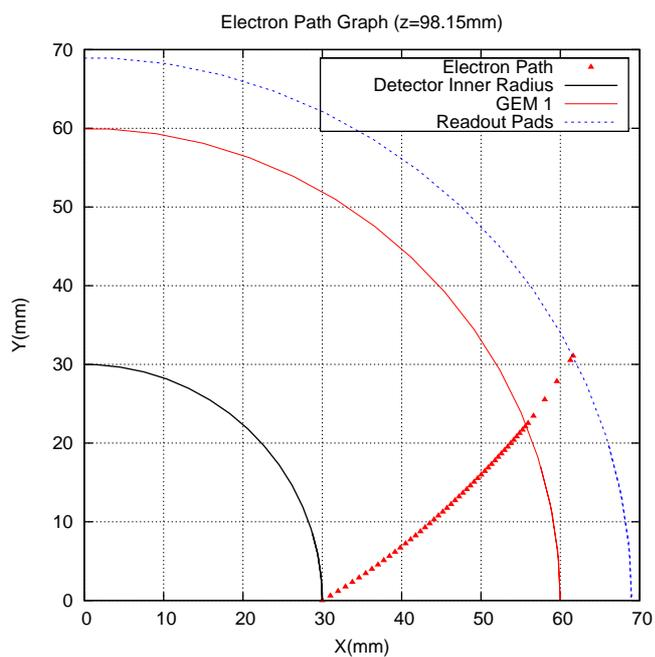
Figure 9: Electron path plot for  $z=98.15$  mm. Note that this path has less curvature than the path at  $z=0.15$  mm since the magnetic field is weaker in the  $z$  direction as a result of the fringe effects near the outer edge of the RTPC.
