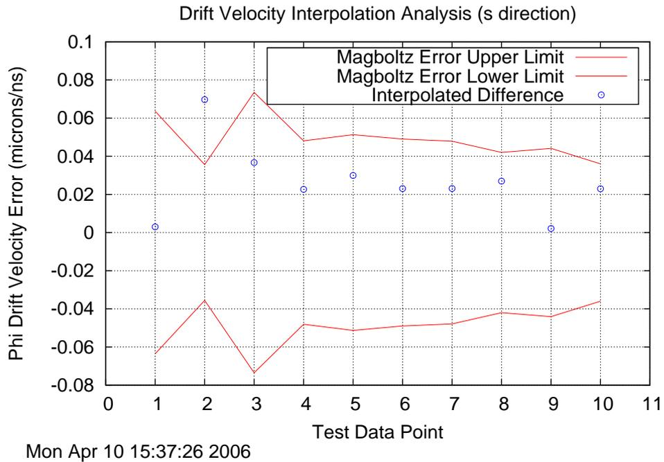
Figure 6: Interpolation Verification:  $s$  direction. The mean Magboltz error was  $0.0491 \frac{\mu m}{ns}$  while the mean interpolated error was  $0.0260 \frac{\mu m}{ns}$ . Since most interpolated errors lie within or very near the Magboltz error range, we can use the interpolation calculation with the current drift velocity map size without contributing significantly to the error.
