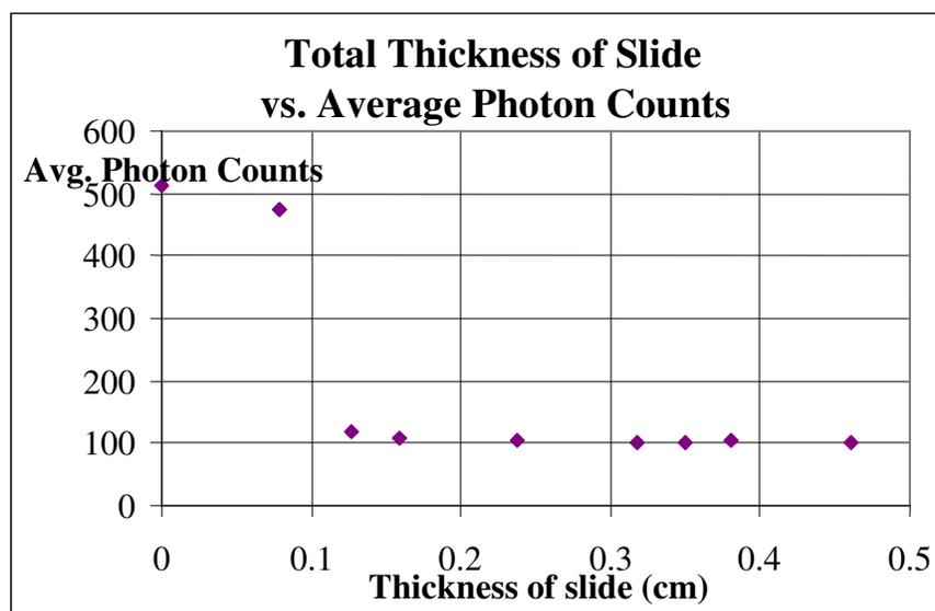
**Figure 15:** Thickness of Slide vs. Average Photon Counts. The first point, at a slide thickness of 0, was taken with no slide between the dot and the camera. The second point, at a slide thickness of 0.08 cm, represents the thickness of only the glass slide, with no paraffin on it. The third data point represents the first slide actually dipped in paraffin.
