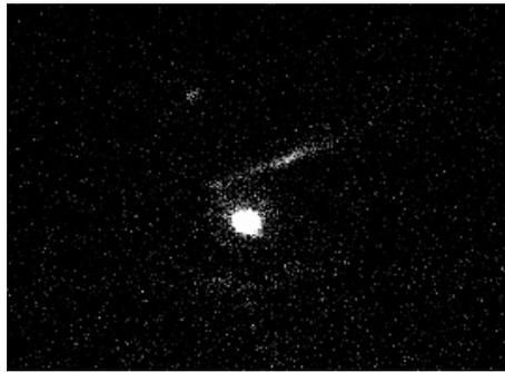
**Figure 12:** Image obtained of quantum dots, utilizing the 800 nm bandpass filter on the camera and a 405 nm bandpass filter on the exciting light source. The rim of the Petri dish is removed and has been covered with black tape to prevent reflection. The small line of the light above the dot in the image, however, is likely a reflection of the edge of the tape covering the Petri dish.
