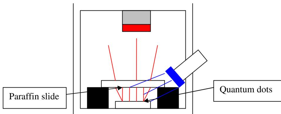
**Figure 13:** A diagram of the set-up used to determine the amount of light from the dots that would pass through various thicknesses of paraffin on a microscope slide. The distance from the dots to the paraffin slide is 6.5 cm. Of note: The exciting light (blue) does not pass through the paraffin slide. Only the emitted (red) light passes through the slide.
