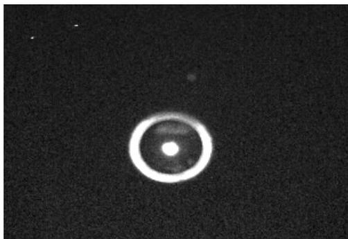
**Figure 11:** Image obtained of quantum dots, utilizing the 800 nm bandpass filter on the camera and a 405 nm bandpass filter on the exciting light source.
