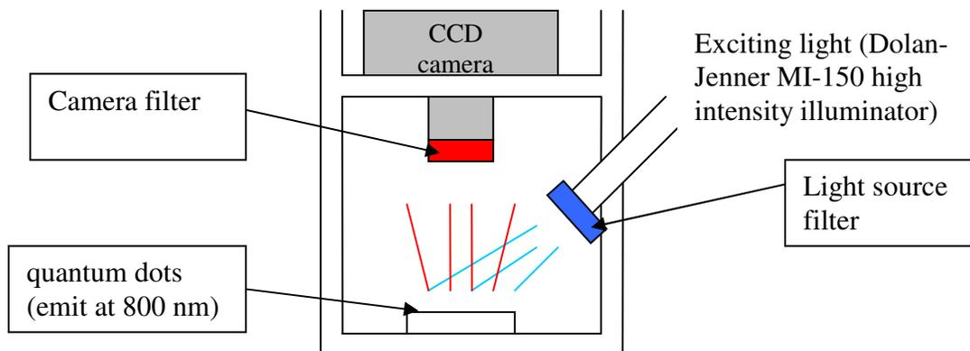
**Figure 9:** Optical Set-up of quantum dot imaging system
