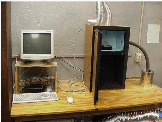
**Figure 6:** The final set-up the liquid nitrogen evaporate cooling system. The liquid nitrogen boils in the metal can and the cold gas passes through the gray foam tube and into the upper chamber of the cabinet, where the camera is located. The cold vapor moves over the camera, drawing heat away, and then leaves the upper chamber through the venting tube at the top.
