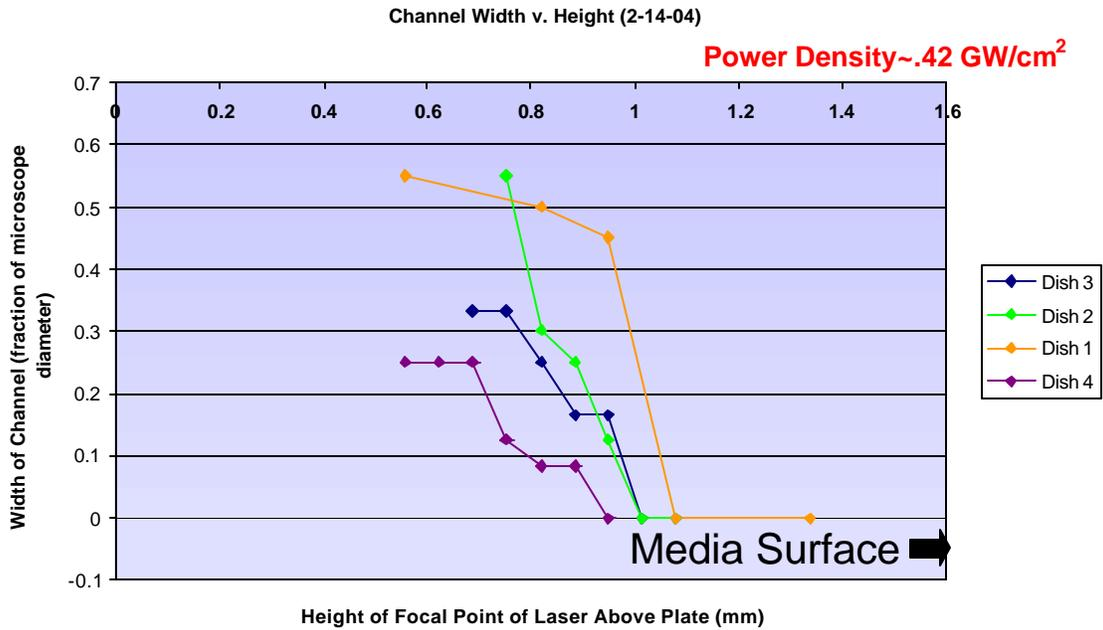
Figure 4: This next set was grown in 4mL of media in each of the 4 culture dishes. The power density of the laser was measured at ~.42 GW/cm<sup>2</sup>.
