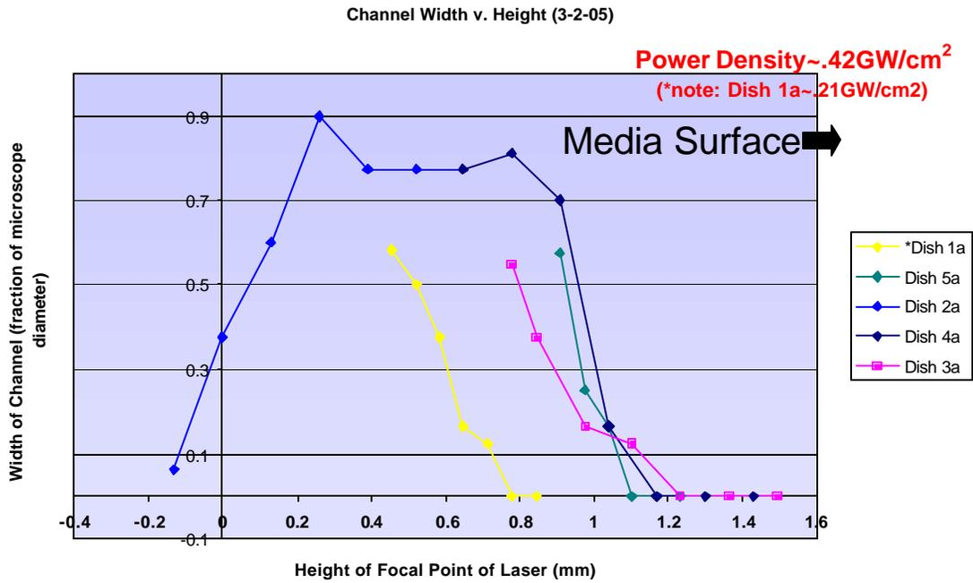
Figure 6: This set was grown in 4mL of media in each of the 4 culture dishes. The power density of the laser was measured at ~.42 GW/cm<sup>2</sup>.
