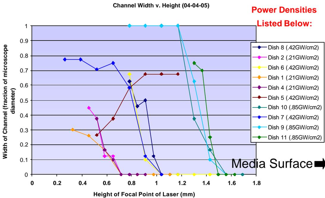
Figure 7: This set was grown in 4mL of media in each of the 11 culture dishes. The power density of the laser was between ~.21 GW/cm<sup>2</sup> to ~.85 GW/cm<sup>2</sup>.
