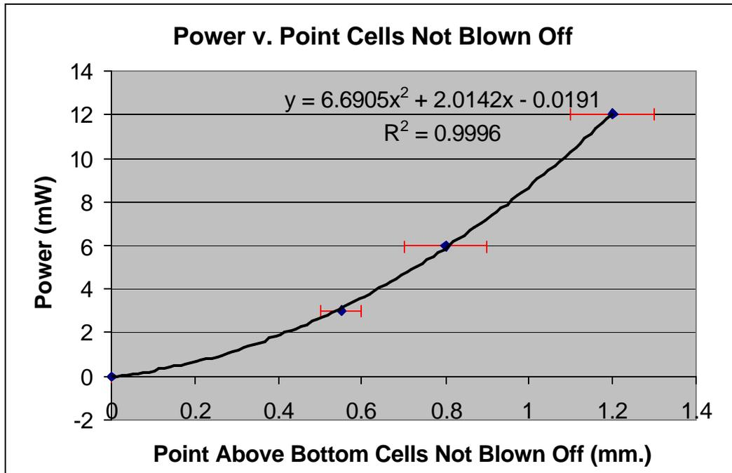
Figure 8: This graph displays the laser power at which cells were no longer blown off. The relationship between these quantities is best modeled by a polynomial form.
