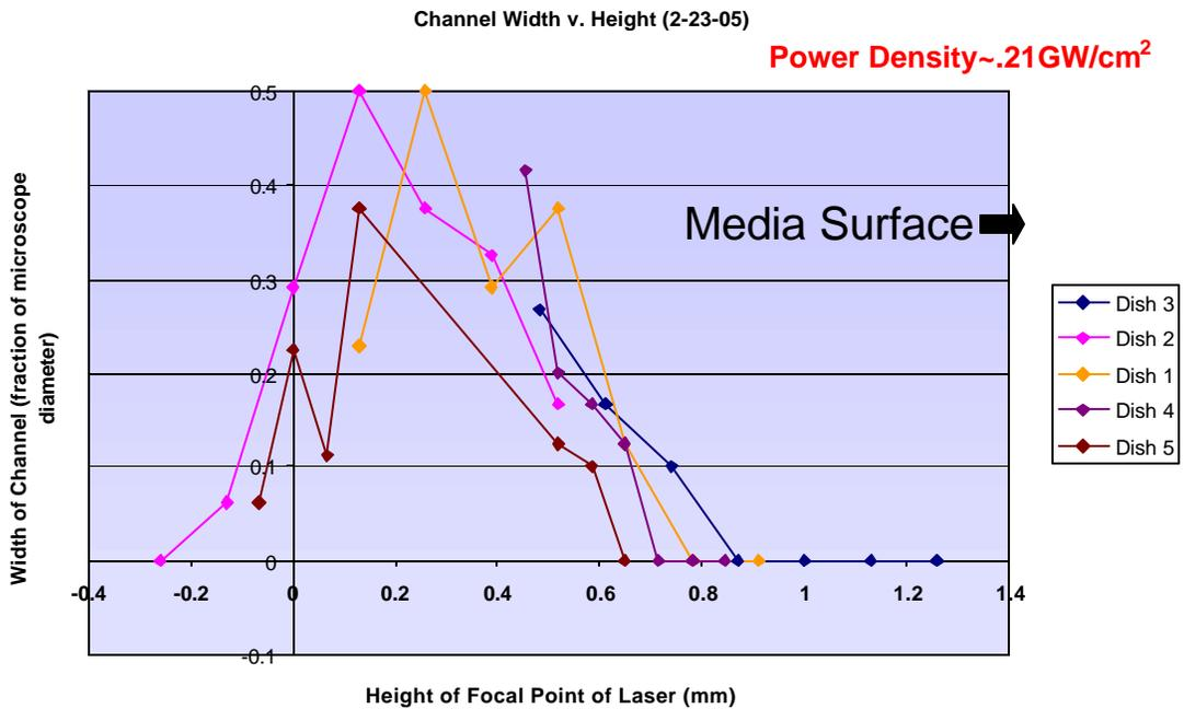
Figure 5: This set was grown in 4mL of media in each of the 5 culture dishes. The power density of the laser was measured at ~.21 GW/cm<sup>2</sup>.
