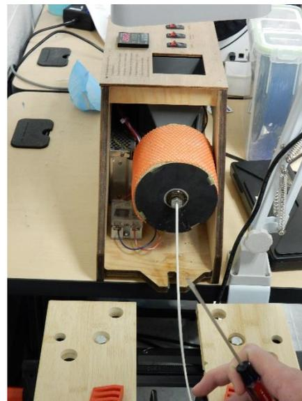
We began to attempt successive extrusions at higher and higher temperatures until we found the correct temperature (a trial and error method). At 160 degrees Celsius we began to observe some extruded filament (all degree measurements will be in Celsius for the remainder of this paper). However, this filament was very brittle, chalky, and clumpy. We speculated that these clumps were unmelted plastic precursor pellets. We increased the temperature, expecting
