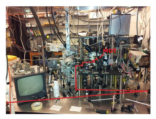
Figure 3.6: Image of the entire optics table. The telescope on the lower section collimates the beam. The beam path is traced.
