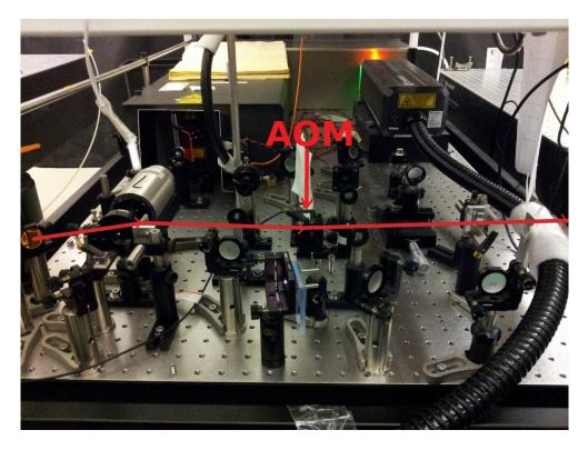
Figure 3.7: Placement of the AOM and cylindrical telescope. The beam path is traced.
