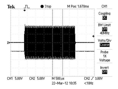
Figure 3.13: Amplitude-modulated RF pulse. The pulse is 3ms long, with a frequency of 700 kHz.
