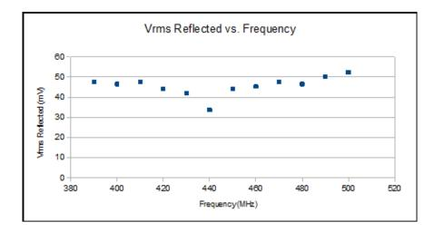
Figure 3.4: Plot of  $V_{rms}$  reflected vs. Frequency. The smallest reflections occur at 440 MHz.
