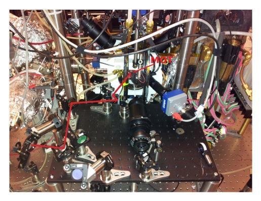
Figure 3.5: Image of the top part of the optics table. The beam path is traced.
