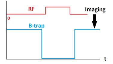
Figure 3.15: Signal representation of when the RF and B-trap are on during procedure. Imaging occurs after the RF is turned off.
