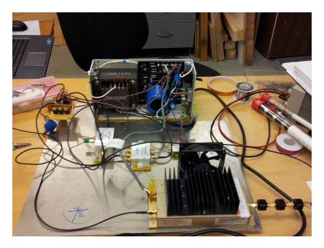
Figure 3.10: The AOM amplifier circuit.
