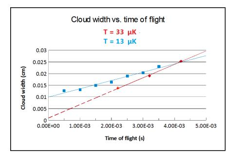
Figure 3.16: Gaussian width vs. time of flight for trapped atoms without adiabatic cooling (red) and with adiabatic cooling (blue). The temperature drops from  $33\mu$ K to  $13\mu$ K.
