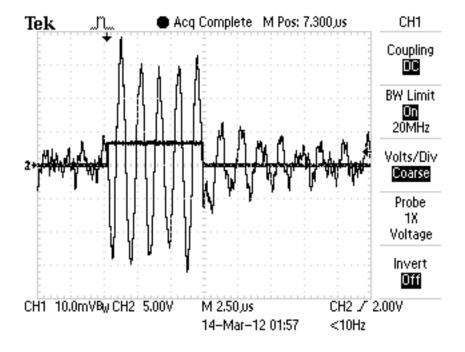
after the burst, possibly caused by reflections of the signal from the vacuum cell.
