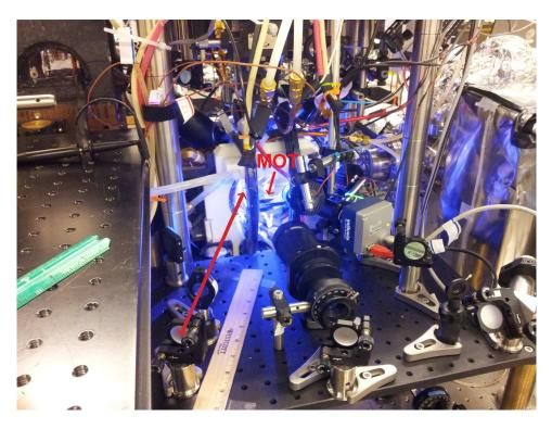
Figure 3.8: The other side of the vacuum cell. The beam is retroreflected to gain more power. The beam path is traced.
