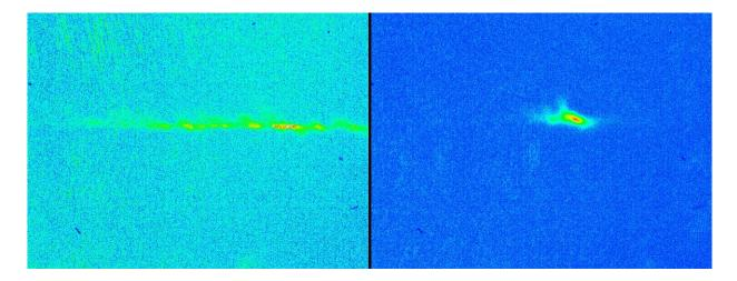
Figure 3.9: Imaged atoms suspended in the dipole trap on the left, and in the latticed dipole trap on the right. The lattice prevents the atoms from axially spreading, keeping them confined to a smaller area.
