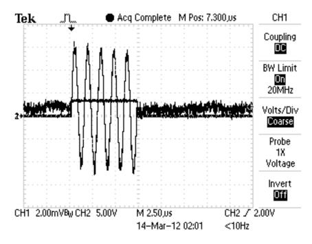
Figure 3.11: RF burst output from signal generator.
