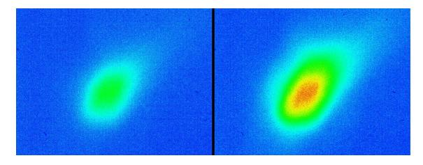
Figure 3.14:  $|F = 2, m_F = +2$ > atoms without optical pumping on the left, with optical pumping on the right. There are significantly more atoms trapped with optical trapping than without.
