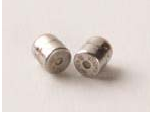
Figure 2: Knowles FG-3329 electret microphones
