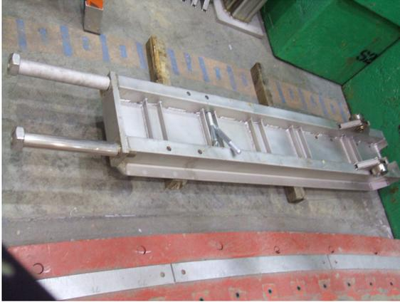
(a) The sliding arms can be seen in the Hall C before being installed. The threaded rods which were used to hold the VDC packages were covered with steel tubes prior to installation. The mounting brackets for the pancake cylinders can be seen in the back right.
