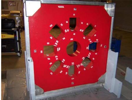
FIG. 3.9: The defining collimator shown before installation. This collimator defines the experimental acceptance for  $Q_{weak}$  [8].
