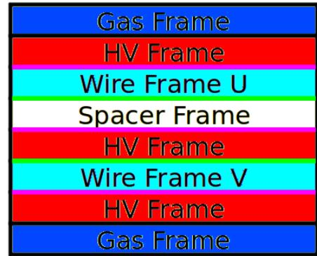
(b) Layering for one VDC. The HV foils are shown in magenta and wire planes are shown in green. The center foil was aluminized foil on both sides to provide field in both cells of the VDC.
