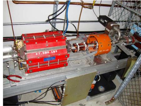
(b) Air-core coils in position on the beamline.
