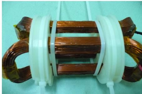
(a) Air-core coil used for driven modulation.
