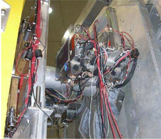
FIG. 3.15: Region II HDCs installed downstream of QTOR in Hall C.
