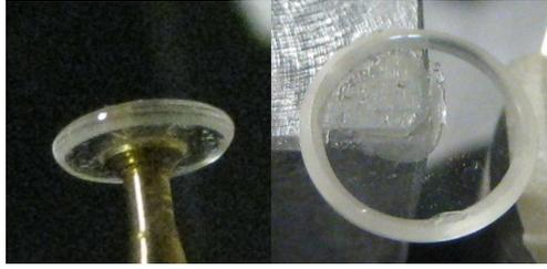
FIG. 2.9: Lithium niobate WGMR disks were  $\sim 7$  mm in diameter and 1 mm thick. *Left:* Disk mounted on brass post for polishing. *Right:* Disk mounted in apparatus for prism coupling.
