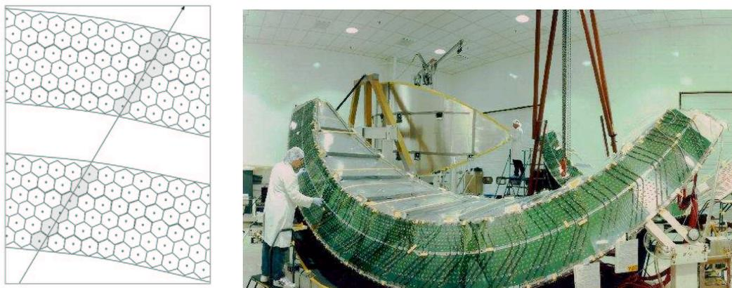
FIG. 3.19: Drift chamber cell configuration with a typical track indicated (left) and photograph of a completed drift chamber sector (right)Ref. [1].
