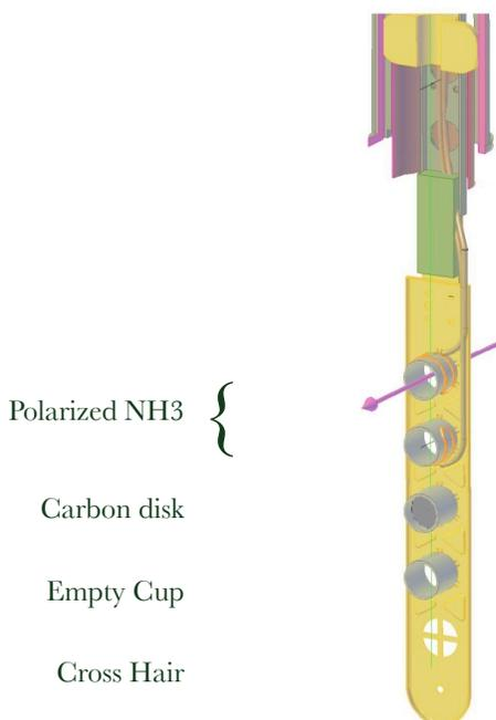
FIG. 3.8: The target stick used during the experiment. The first two cups contained ammonia and the third had a carbon disk. The last one was left empty for background studies. The cross-hairs at the bottom were used to align the beam on the target.
