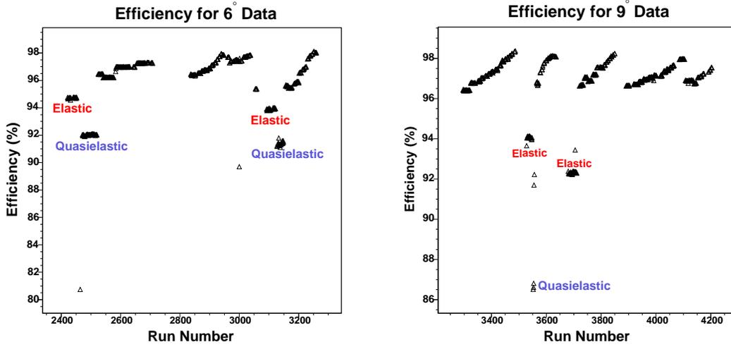
FIG. 7.1: The 1-track efficiency per run for the  $6^\circ$  (left) and  $9^\circ$  (right) data.
