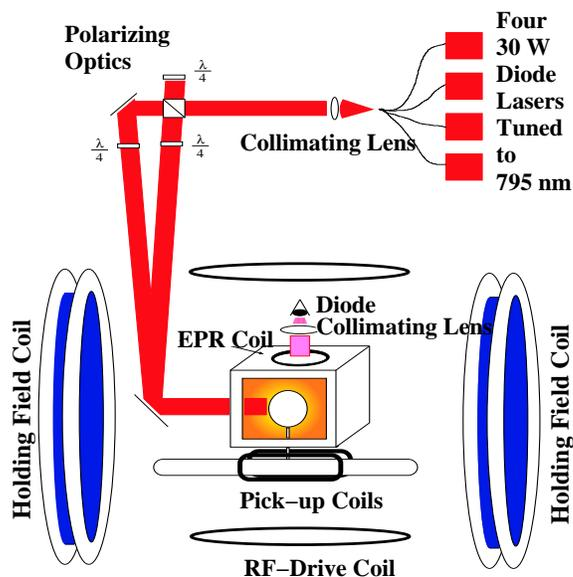
FIG. 5.9: Diagram of the polarized  $^3\text{He}$  Target system. The transverse Helmholtz coils are not shown to provide clarity.
