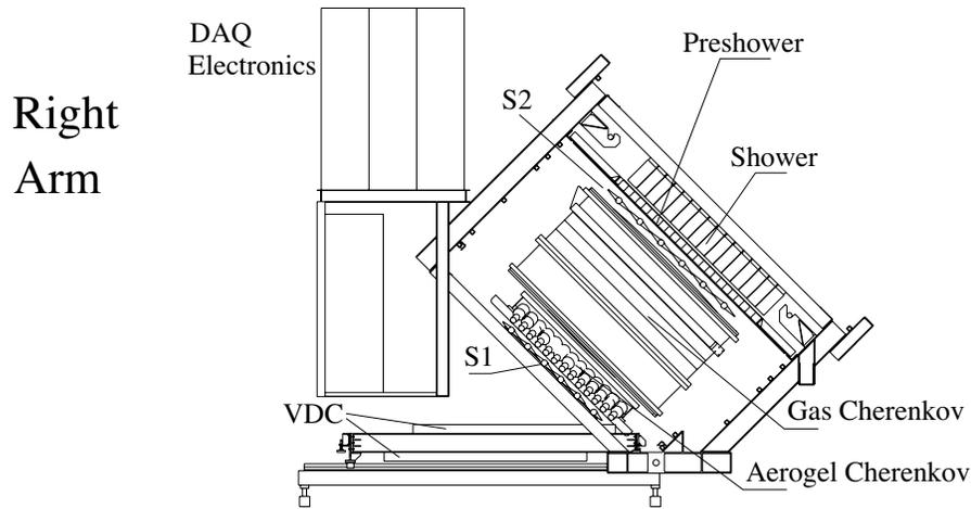
FIG. 6.3: Detector package for HRS-R. Note the aerogel Čerenkov was not used or present in the detector stack during E97-110. Reproduced from [67].
