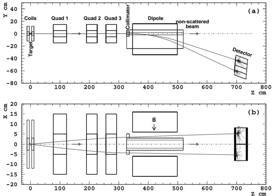
FIG. 5.7: Schematic of the Møller Polarimeter with the top plot presenting a side view and the bottom a top view. Reproduced from [67].
