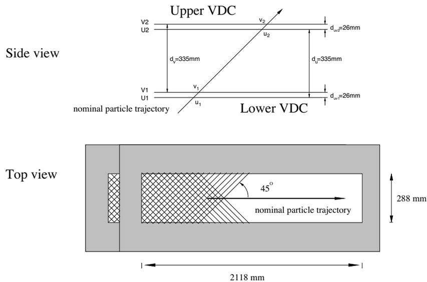
FIG. 6.4: Schematic diagram of the Hall A vertical drift chambers. Reproduced from [67].
