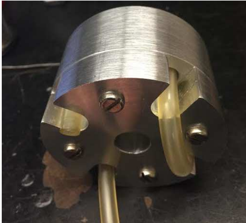
Figure 2: The rubidium cell holder
