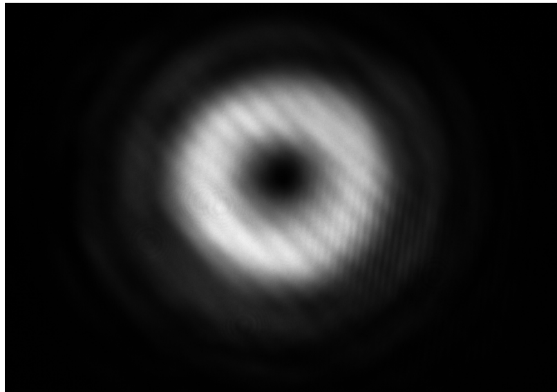
Figure 4.1: An example of a raw image of camera output. Here, interference is visible as a stripe pattern overlaid upon the beam.
