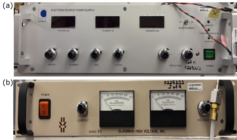
Figure 3.3: Electron beam controllers. (a) Filament source controller for energy, emission current, and steering. (b) Voltage source.
