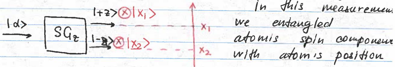
Quantum state after  $SG_z$ :  $c_1|+z\rangle \otimes |x_1\rangle + c_2|-z\rangle \otimes |x_2\rangle$
