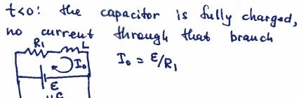
to: once the switch is closed, current will start flowing, discharging the capacitor, and transferring the stored electrical energy from the capacitor to the inductor and then back — oscillating circuit. However, singe energy is lost at the resistor, the oscillations decay.
