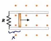
The figure shows a top view of a bar that can slide without friction. The resistor is  $R=6.0~\Omega$ , and a magnetic field  $B=3.20~\mathrm{T}$  is directed out of the page and fills the whole area. The length of the bar is  $l=1.20~\mathrm{m}$ .
