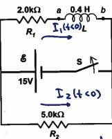
a) What are the steady-state (t < 0) currents in the resistors  $R_1$  and  $R_2$ ?
