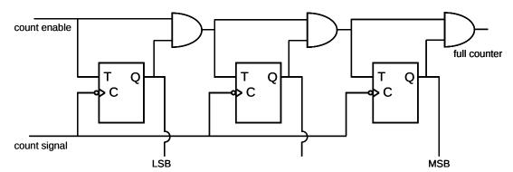
**Figure 3:** 3-bit synchronous counter circuit with T-type flip-flops. The counter reset-to-zero feature shown in figure 2 has been omitted for clarity.
