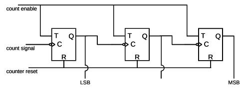
Figure 2: 3-bit ripple counter with reset-to-zero and count enable features.
