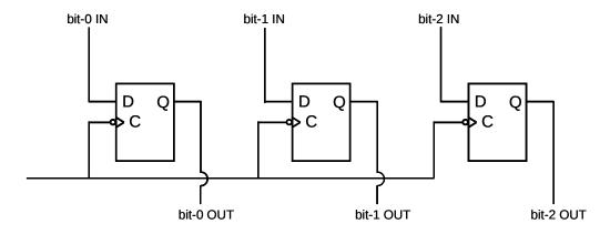
Figure 4: Circuit diagram for a 3-bit PIPO-type register.
