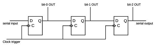
Figure 5: 3-bit FIFO-type shift register with a parallel out read option.
