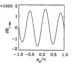
FIG. 5. The normalized, radial, vacuum magnetic perturbation, calculated at r=c, which generates the locking potential (117).
