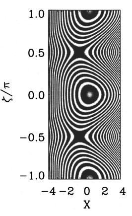
FIG. 2. Island flux surfaces calculated from Eq. (101), using the parameters listed in Table I. The stability index for the fundamental harmonic takes the value  $E_1 = 5$ .
