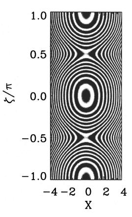
FIG. 3. Island flux surfaces calculated from Eq. (101), using the parameters listed in Table I. The "skew" term has been neglected. The stability index for the fundamental harmonic takes the value  $E_1 = 10$ .
