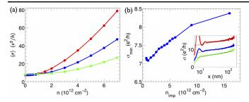
FIG. 1 (color online). (a)  $\langle \sigma \rangle$  as a function of n for  $n_{\rm imp} = (3,5,9) \times 10^{12} \ {\rm cm}^{-2}$  from top to bottom. (b)  $\langle \sigma \rangle$  at the DP as a function of  $n_{\rm imp}$  for the case of Coulomb disorder. The inset shows  $\langle \sigma \rangle$  as a function of sample length  $L \equiv x$  for W = 160 nm, and  $n = (3,2,1) \times 10^{12} \ {\rm cm}^{-2}$  from top to bottom. The dashed lines show  $d\sigma/d \ln L = 4e^2/\pi h$ .
