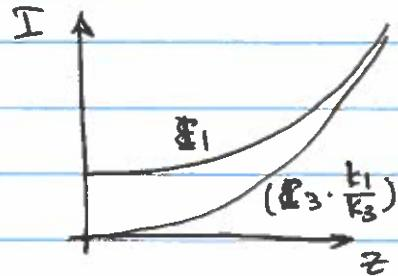
Both fields grow exponentially and simultaneously until the pump is depleted
