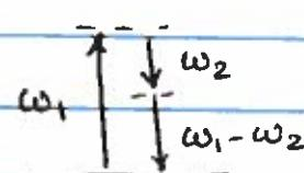
Parametric down conversion : pair of field is generated
