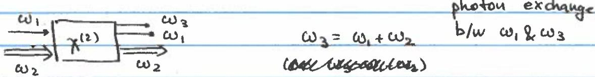
Strong  $\omega_2$  - pump,  $\omega_1$  - signal,  $\omega_3$  - idler
