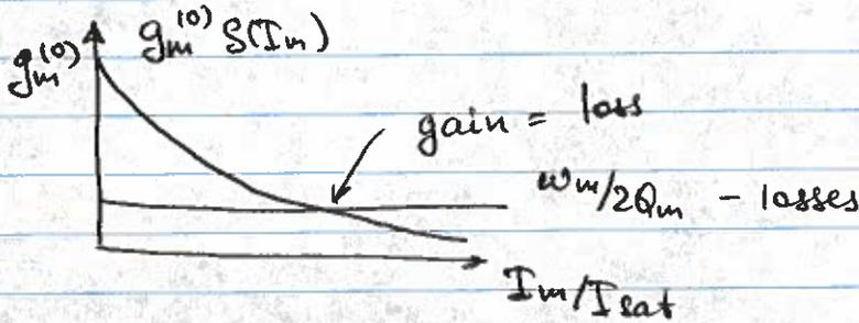
Small intracavity intensity  $\rightarrow$  large gain (field strengthens)
