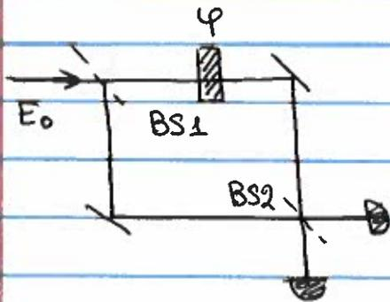
Objective - to measure the phase shift  $\varphi$
