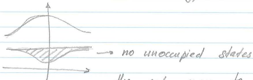
the only way to produce electric current is to zap the material with enough energy to push electrons to the excited band ( $\Delta E > \text{bandgap}$ )
