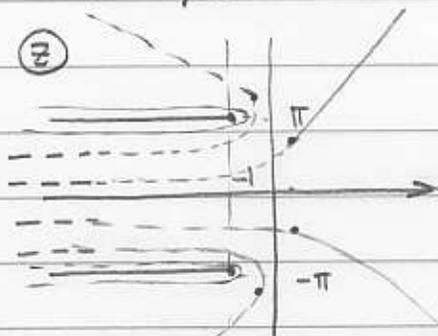
Equipotential lines at the edge of the capacitor (of water flow out of the straight tube)
