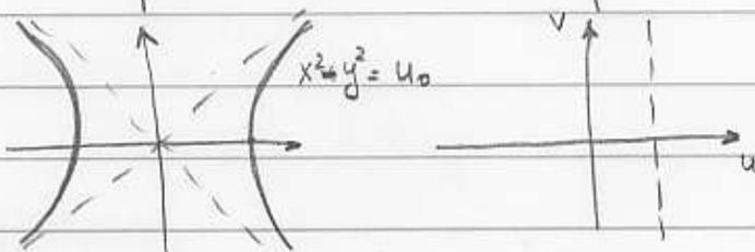
Each quadrant of  $z$ -space is mapped into a semi-plane in  $w$ -space. Thus, the complex plane in  $z$ -space is mapped into two folds of  $w$ -space (separated by  $2\pi$  phase).
