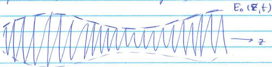
$$\begin{aligned} \frac{\partial E}{\partial t} &= \frac{\partial}{\partial t} \left( \frac{1}{2} \vec{E}_0(z, t) e^{ikz - i\omega t + i\varphi(z, t)} \right) \\ &= \cancel{\left[ (-i\omega) \vec{E}(z, t) + \frac{1}{2} \frac{\partial \vec{E}_0}{\partial t} e^{ikz - i\omega t + i\varphi} + \vec{E}(z, t) i \frac{\partial \varphi}{\partial t} \right]} \end{aligned}$$
