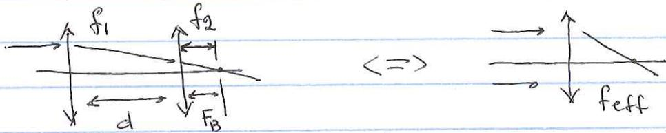
$$\frac{1}{f_{\text{eff}}} = \frac{1}{f_1} + \frac{1}{f_2} - \frac{d}{f_1 f_2}$$
