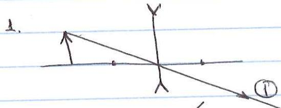
Beam travels through the center of the lens with no change
