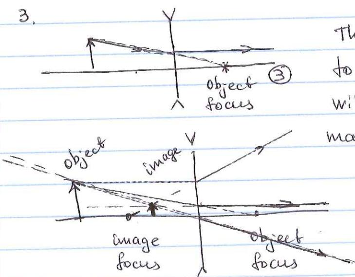
The beam that aims to the object focus will go parallel to the main axis after the lens
