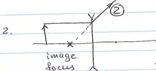
The beam traveling parallel to the optical axis, after the lens will continue as if it originates from an image focus.
